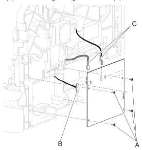
Replacement Warning: When replacing the HVPS card assembly, ensure that the two high voltage connections (C) are properly replaced.
