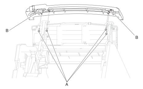
4. Remove the operator panel latch assembly.
