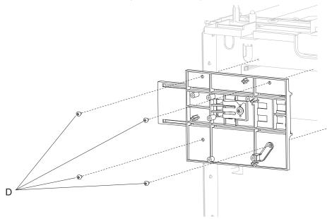
6. Remove the card mount option with the media size actuator.
