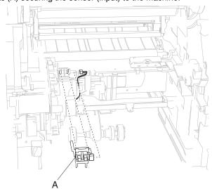
3. Remove the sensor (input).
