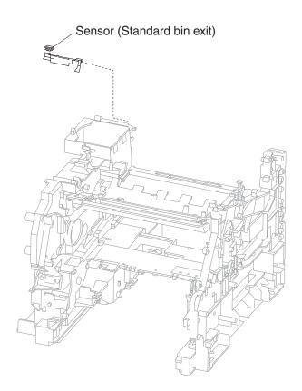
The standard media exit ejects printed media from the printer to the standard bin .
