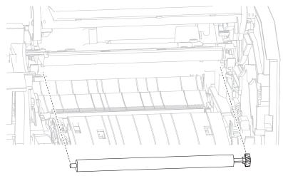
Replacement Warning: When replacing the transfer roll assembly, do not touch the foam surface.
