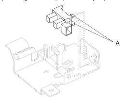
3. Remove the sensor (duplex input).
