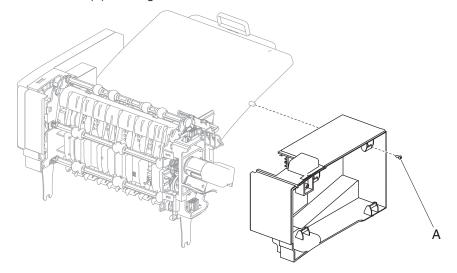
3. Holding the rear of the left inner cover, pull out while simultaneously separating it from the option.
