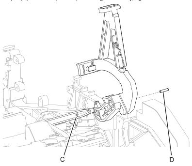
6. Remove the operator panel hinge assembly, right.
