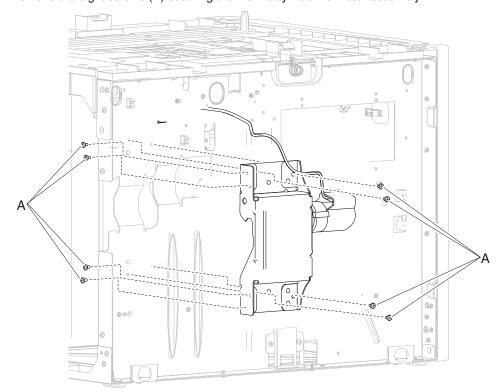
5. Remove the HCIT tray lift drive motor assembly.
