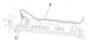
Replacement Warning: When replacing the duplex drive motor assembly, ensure that all harnesses are properly re-routed.
