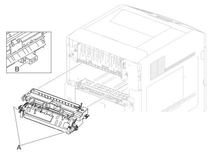
Replacement Warning: When replacing the fuser unit assembly, ensure that the electrical connection (B) and the two buttons (A) are properly secured.
