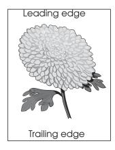
The printed image is not paralleled with both sides of the media.
