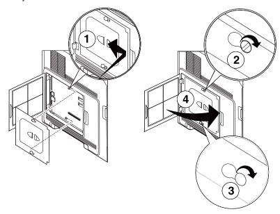
15. Lift the printer off the 250/550 sheet optional drawer, place the RFID option on top of the drawer, and place the printer on top of the RFID option.
