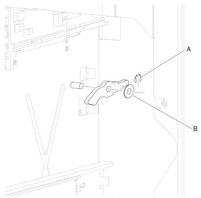
3. Remove the HCIT tray closed latch with spring.
