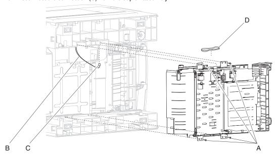
Note: When removing the duplex assembly, the lower duplex drive belt (D) will become detached.
