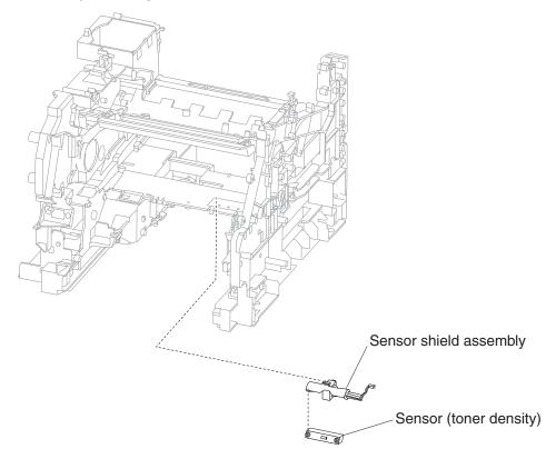
The image density sensor assembly uses a reflection type sensor that detects a pre-placed toner patch and image on the photoconductor (drum) and outputs pulses when the central line of the patch image aligns with the central line of the detector. The sensor outputs pulses at the timing the patch image passes the sensor. Therefore, observing changes of intervals at which pulses are output leads to toner density detection.
