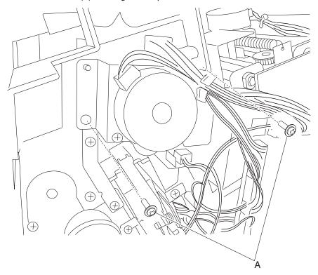
5. Remove the paddle drive motor assembly.
