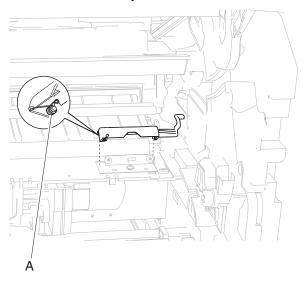
3. Remove the sensor shield assembly.
