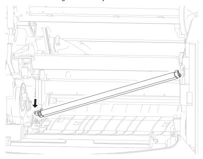
4. Detach the right side of the charge roll assembly from the machine.
