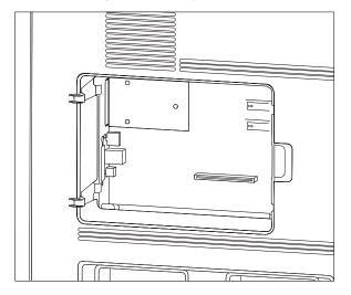
8. Snap the plastic tee card holder into place on the system board.
