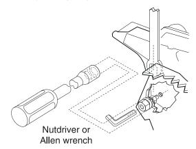
4. Install the new alignment assembly. Turn the reference screw clockwise with a 7 mm nut driver or M3 Allen wrench until it touches the back of the reference plate, and tighten the nut with a 5.5 mm wrench.
