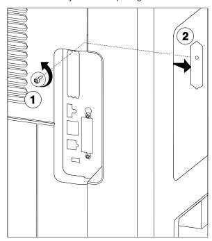
7. Locate the interface card mounting area on the system board.
