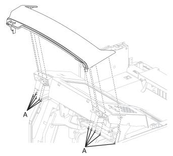
3. Remove the operator panel cover latch assembly.
