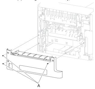
4. Remove the cover assembly, rear lower.
