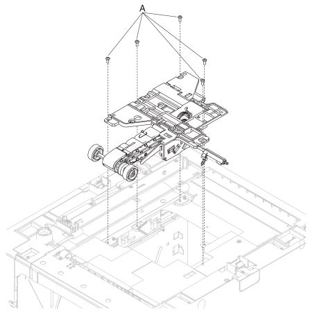
5. Remove the HCIT pick arm bracket assembly from the drawer by slightly lifting and removing it.
