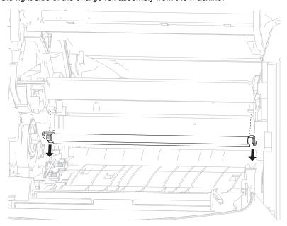
5. Remove the charge roll assembly.
