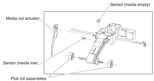
Since all media trays are functionally equivalent in terms of the switch (media size), sensor (media empty), sensor (media low), only the components of one tray are described here.
