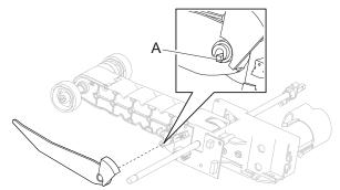
3. Remove the 250-sheet media out actuator from the drawer.
