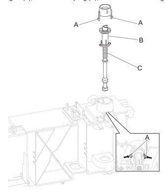
4. Remove the 550-sheet option drive shaft with spring.
