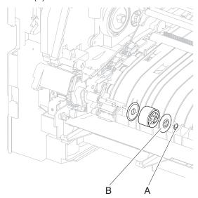
4. Remove the MPF pick roll assembly.
