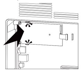
11. Insert the long thumbscrew into the hole in the interface card. Turn it just enough to hold the card in place. Do not tighten yet.
