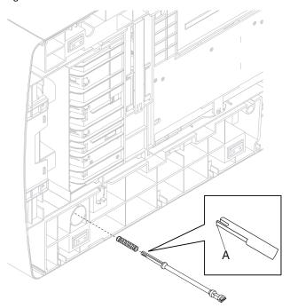
**Replacement Warning:** When replacing the option drive shaft, ensure that the plastic hook (A) is not damaged, or the option drive shaft will not remain secured.
