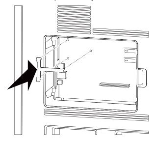
9. Angle the interface card through the connector opening.
