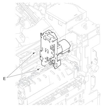
9. Remove the redrive motor assembly.
