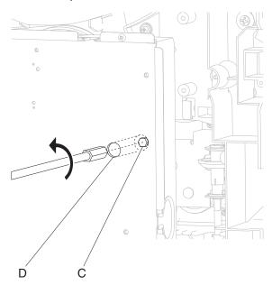
Replacement Warning: When replacing the alignment assembly, ensure that the media skew is properly adjusted using the adjuster screw (C) or jamming will occur. Go to "Alignment assembly adjustment" on page 4-4.
