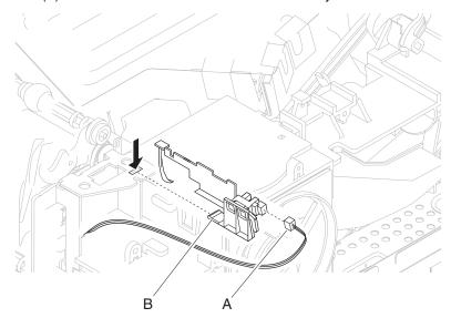
4. Remove the standard bin actuator assembly.
