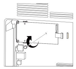
12. Insert the screws to secure the mounting bracket to the system board.
