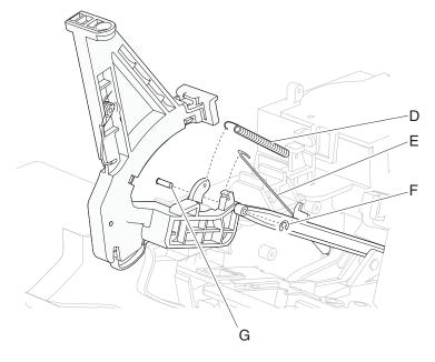
10. Remove the operator panel hinge assembly, left.
