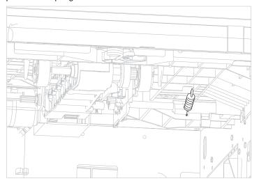
4. Remove the five screws (A) securing the HCIT pick arm bracket assembly.
