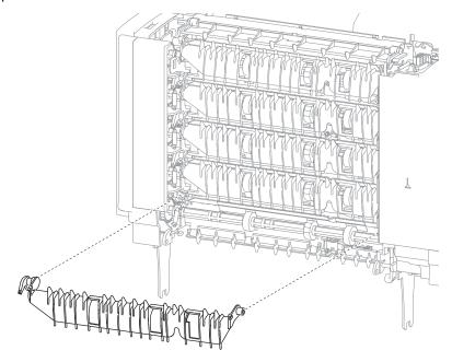
Replacement Note: The static brush mylar assembly is attached to the media bin fifth deflector. Do not forget to reinstall it on the new deflector.
