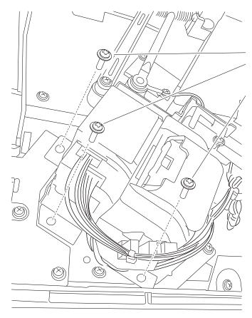
4. Remove the stapler unit assembly.
