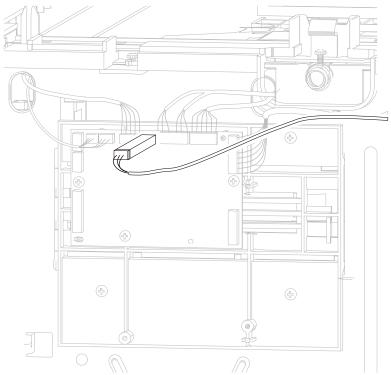
**Note:** Remove the cable restraint, and observe the routing for reinstallation.
