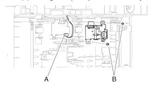
5. Remove the duplex input sensor assembly.
