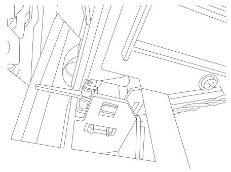
Replacement Notes: Using needlenose pliers, place the rear most tab in the sensor bracket first. Then push on the rear face of the sensor until the other two tabs snap into place.
