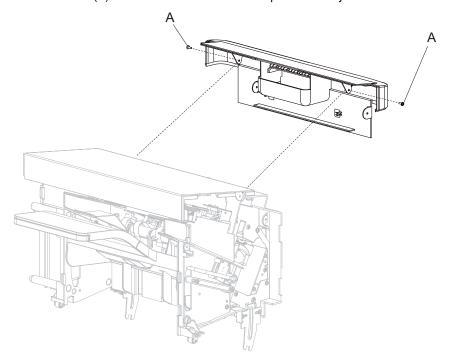
3. Lift up and to the rear to remove the cover.
