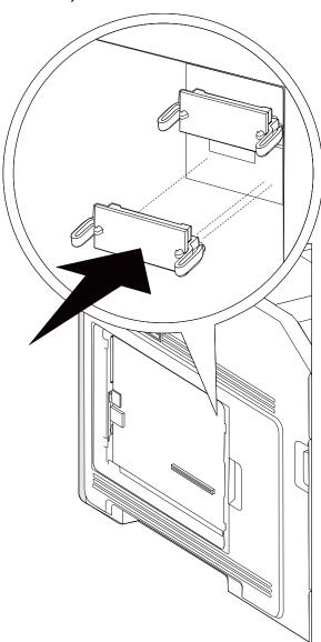
6. Remove the metal cover from the system card opening.
