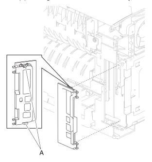
4. Remove the connection bezel assembly, rear.
