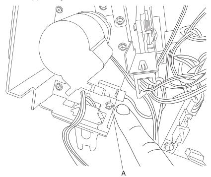
Note: The tabs may be difficult to access. The use of a spring hook or flat-blade screwdriver may be necessary to release the tabs.
