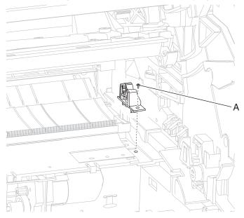
4. Remove the transfer roll bracket assembly, right.
