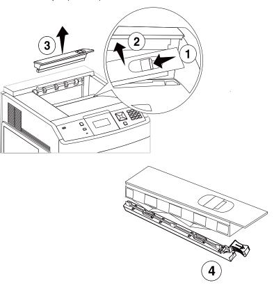
18. Install the new wiper. Turn the printer on.
