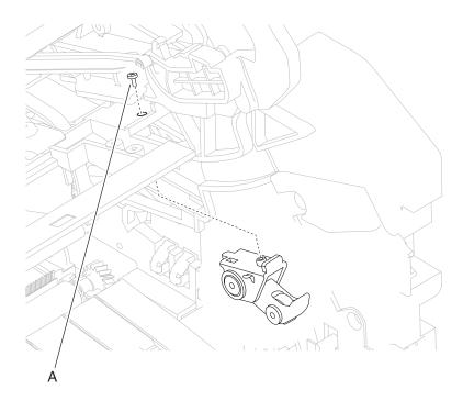
3. Remove the print cartridge clamp assembly.
