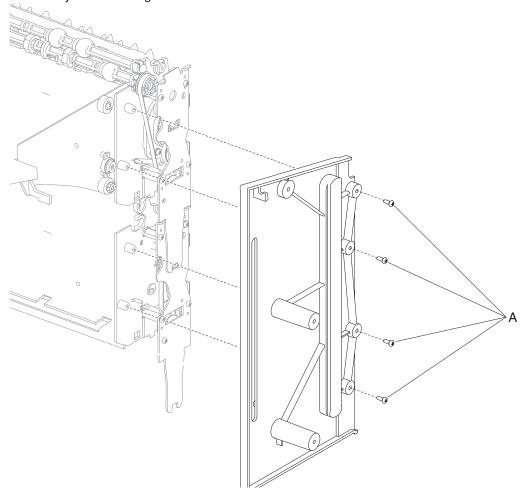
Note: When installing the right frame, make sure the media output bin assembly is aligned properly.
