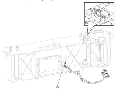
4. Remove the upper interface cable assembly.
