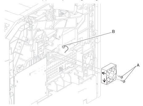
Replacement Warning: When replacing the print cartridge cooling fan, ensure that it is installed as shown in the picture.
