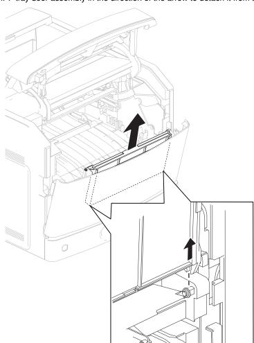
5. Slide the MPF tray door assembly in the direction of the arrow to detach it from the machine.
