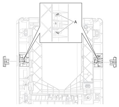
3. Remove the anti-tip latch assembly.
