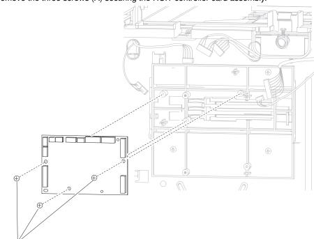
3. Remove the three screws (A) securing the HCIT controller card assembly.
