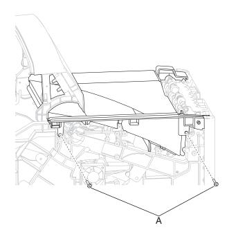
WARNING: When removing the laser cover, ensure that the standard bin actuator assembly does not become damaged.
