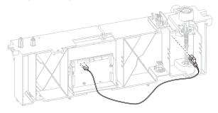
3. Remove the sensor (pass through) with cable.
