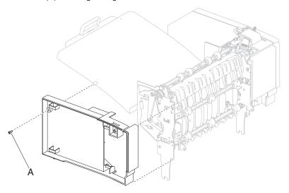
3. At the rear of the right inner cover, pull out from the option and remove the right inner cover.
