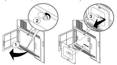
4. Install the firmware card into the system board.
