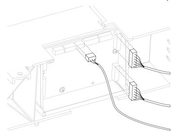
3. Remove the three screws (B) securing the 250-sheet controller card assembly to the 250-sheet frame.
