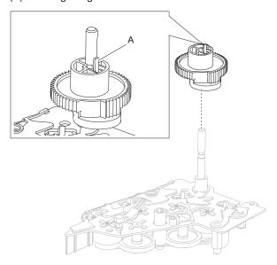
3. Remove the MPF cam gear.
