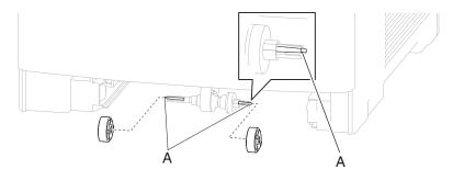
3. Remove the two pick roll assemblies.
