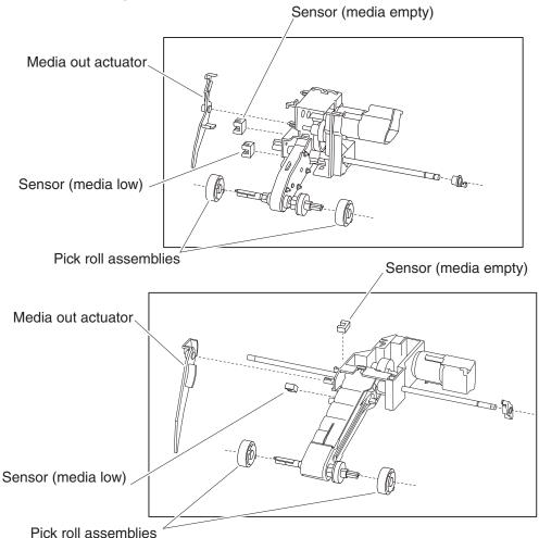
Since all media trays are functionally equivalent in terms of the switch (media size), sensor (media empty), sensor (media low), only the components of one tray are described here.
