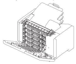
2. Pry the rear door hinges out of the bottom hinges and remove.
