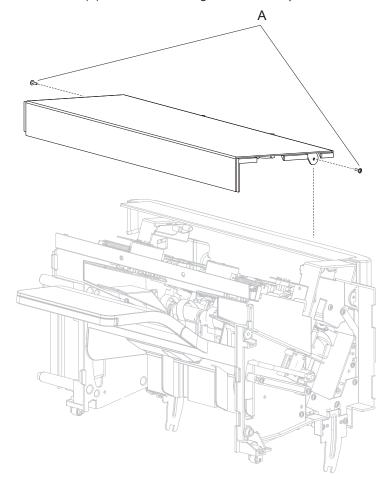
3. Pull up and toward the front to remove the top cover.
