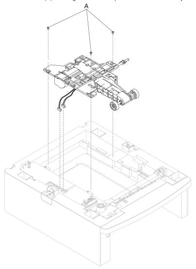
5. Remove the 550-sheet pick arm bracket assembly.
