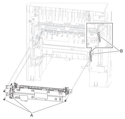
Note: When removing the duplex drive motor assembly, the upper duplex drive belt (B) will become detached.
