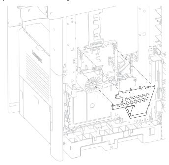
8. Disconnect the USB cable and the cover closed interlock switch harness.
