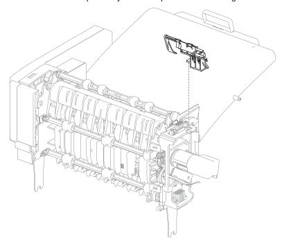
3. If replacing the bracket, remove the sensors (media bin full) from the bracket.
