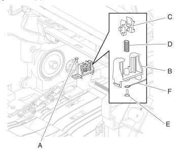
Replacement Warning: When reinstalling the transfer roll bracket assembly, left, ensure that the bushing (C), spring (D), and ground wire (F) are properly replaced.
