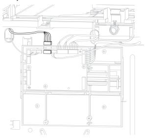
**Note:** Remove the cable from the restraint, and observe the routing for reinstallation.
