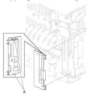
4. Remove the connection bezel assembly, rear.
