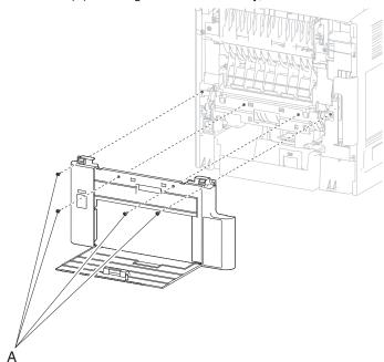
3. Remove the cover assembly, rear lower.
