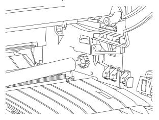
4. Remove the transfer roll assembly.
