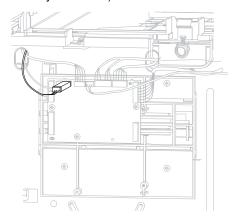
**Note:** Remove the cable from the restraints, and observe the routing for reinstallation.
