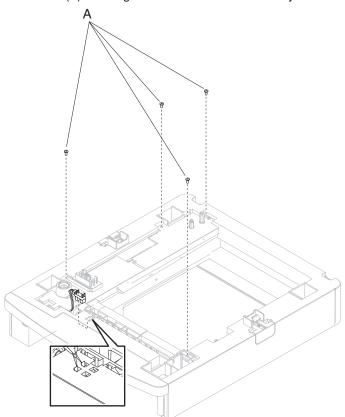
5. Remove the 250-sheet frame assembly.
