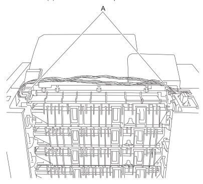
4. Pull the left side up first and carefully unroute the cables from the channels and then remove the top cover.
