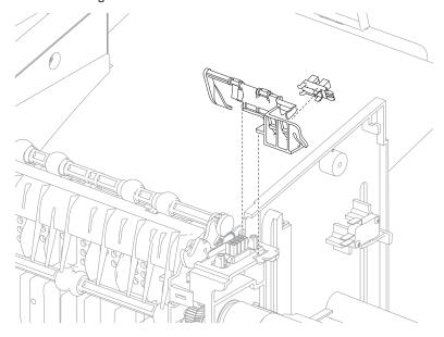
3. Remove the bracket from the frame and disconnect the sensor (media bin full) and media bin full actuator.
