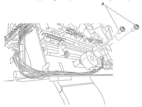
5. Remove the tamper drive motor assembly.
