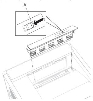
2. Remove the fuser wiper cover assembly.
