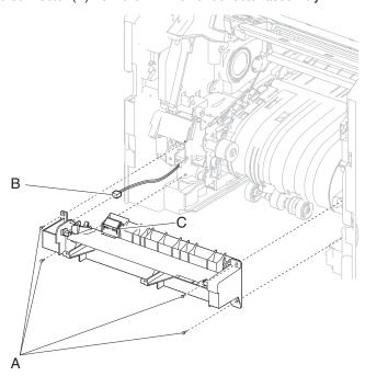
5. Remove the MPF lift plate assembly.
