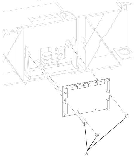
4. Remove the 550-sheet controller card assembly.
