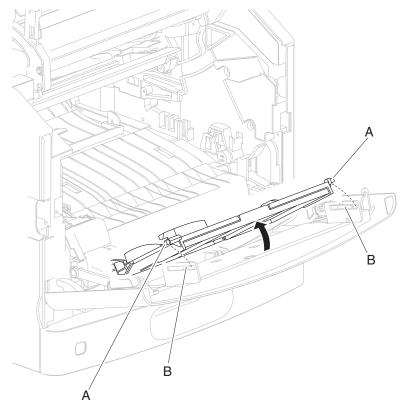
4. While holding the MPF tray in its uppermost position, swing the MPF tray door assembly away from the machine to detach the MPF tray from the machine.
