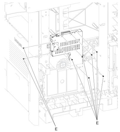
7. Remove the printer controller card cage cover.
