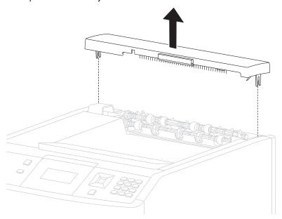
2. Remove the output cover assembly.
