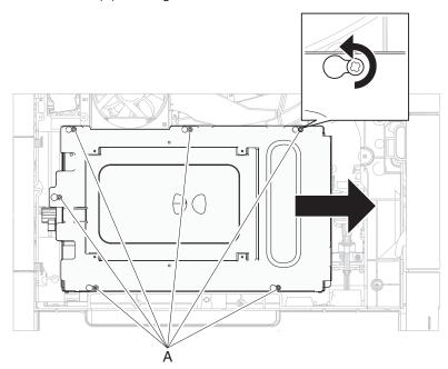
3. Slide the metal shield in the direction of the arrow.
