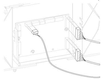
3. Remove the three screws (A) securing the 550-sheet controller card assembly to the 550-sheet frame.
