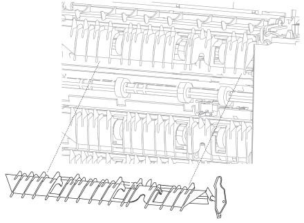
Replacement Note: The static brush mylar assembly is attached to the media bin fifth deflector. Do not forget to reinstall it on the new deflector.
