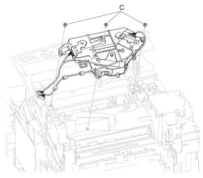
6. Remove the printhead assembly.
