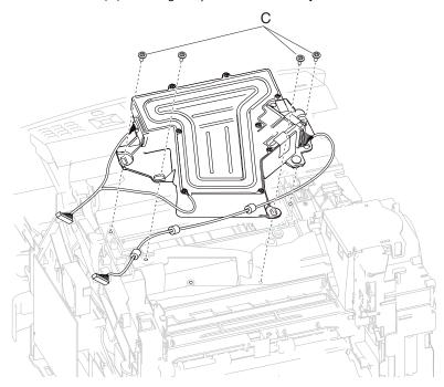
6. Remove the printhead assembly.
