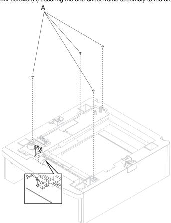
5. Remove the 550-sheet frame assembly.
