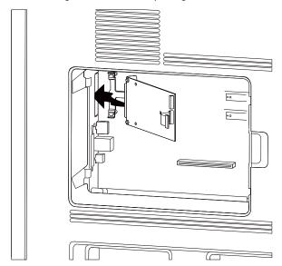
10. Insert the interface card into the plastic tee card holder.
