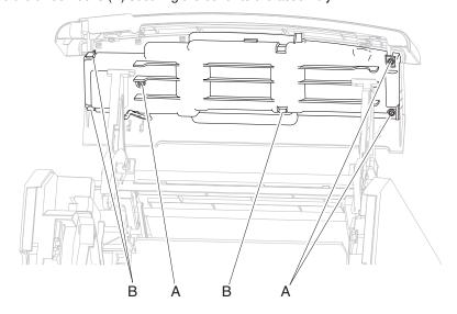
4. Detach the operator panel door assembly from the machine.
