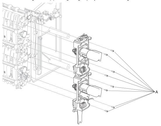
3. Pull the bracket up and let it rest on the assembly with the cables intact.
