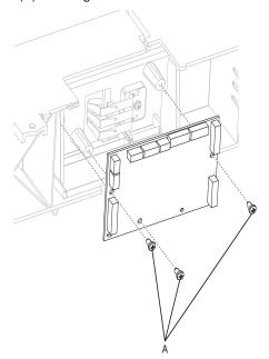
4. Remove the 250-sheet controller card assembly.
