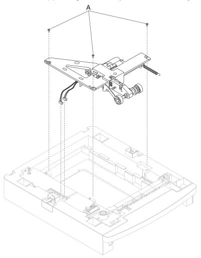
4. Remove the 250-sheet pick arm bracket assembly.
