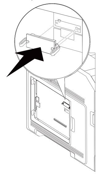
5. Install the flash card into the system board.
