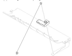
9. Remove the duplex guide assembly, rear.
