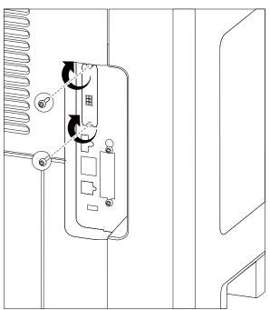
13. Tighten the thumbscrew, and insert the interface card plug into the blue connector on the system board.
