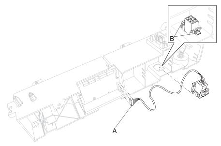
4. Remove the lower interface cable assembly.
