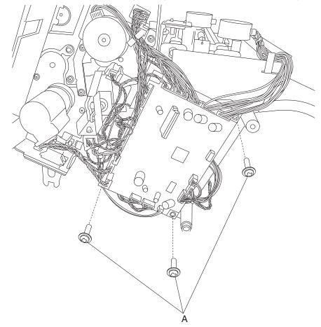
4. Remove the stapler/stacker controller card assembly.
