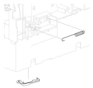
**Note:** The tray roller catch assembly should be removed from the media tray cabinet.
