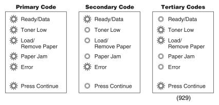
Either the printer's toner sensor is faulty or the print cartridge is defective.
