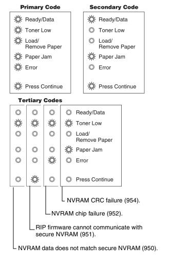
Note: NVRAM is on the operator panel printed circuit board (PCB) while secure NVRAM is on the controller PCB. Check margin alignments after replacing the operator panel assembly. See "Printhead assembly" on page 4-2 (steps 1 through 11) for more information. If margin errors are unacceptable, corrections can only be made through software. Contact the next level of support or Lexmark at 1–800–539–6275.
