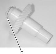
4. Insert the bottom portion and press or pull into position. Note: You should hear two distinct snaps. If you only hear one, the bevel gear is only partially engaged and you should continue to press until the second snap is heard. Very firm pressure is required.
