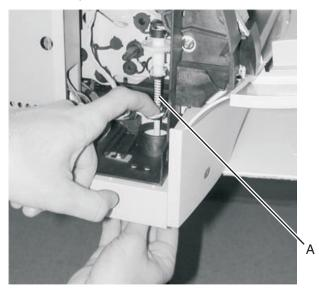
5. Place your thumb on the top of the gear and press firmly down and away.
