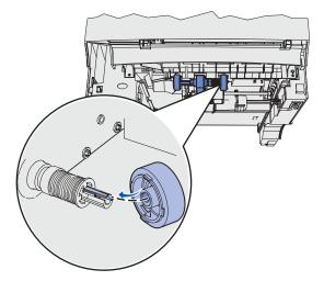
4. Push the pick roller onto the arm with the tab aligned. Repeat this step on the other side to install the other pick roller.
