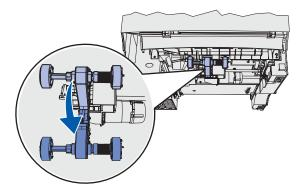
Press on the end of the tab and pull the pick roller off the arm. Repeat this step for the pick roller on the other side. Next, gently release the pick roller arm. Discard the used pick rollers. Remove the new pick rollers from their packaging.
