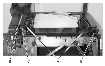
8. Remove the upper front cover hinge assembly.
