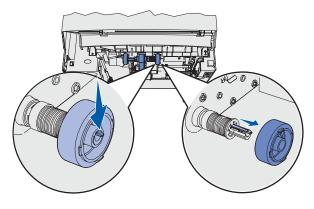
3. Pull the pick roller arm down. Locate the recessed area on the pick roller and align it with the tab on the arm. There are two arrows on each pick roller. Make sure the bottom arrow faces you as you align the recessed area with the tab.
