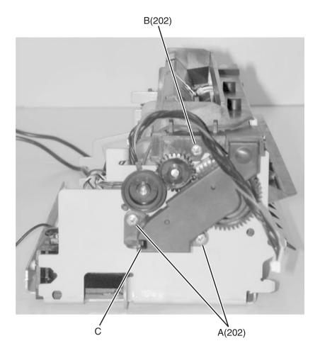
**CAUTION:** Take care when removing the screw, as the lamp is under pressure. When the contact is released, damage to the lamp or contact may occur.
