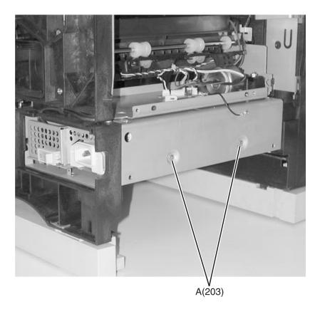
3. Pull the LVPS assembly from the right side of the printer.
