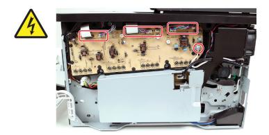
**4** Cut the cable tie, and then remove the four screws.
