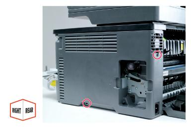
**2** Slightly move the cover to remove the screw behind it.
