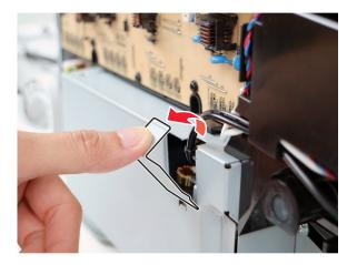
7 Disconnect and release the cables (C), and then remove the two screws.
