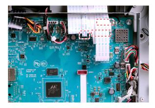
8 Disconnect the cables, and then release the spring (A).
