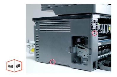
**5** Position the printer as shown, and then release the rear latches.
