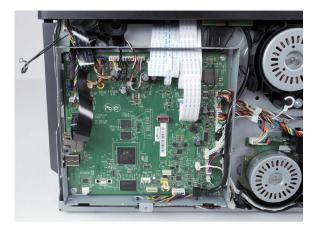
**4** Release the antenna card from its bracket, and then release it from the controller board frame.
