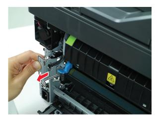
**10** Press the latch. Lock the latch position using a prying tool or screwdriver.
