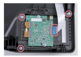
**7** Remove the control panel.
