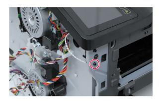
**8** Remove the screw, and then release the switch from its bracket.
