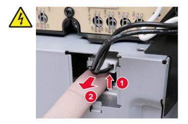
**12** Thread the cable through the hole.
