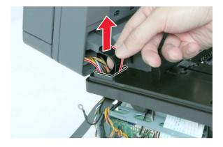
**8** Detach the hinge, and then remove the scanner.
