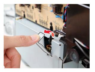
**3** Disconnect all the cables, and then remove the cable screw.
