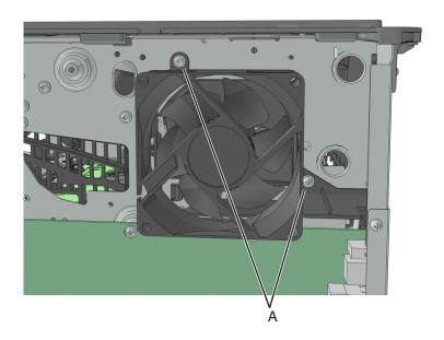
**5** Remove the two screws (B) securing the fan to the fan mount.
