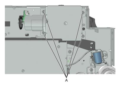
**3** Disconnect the cable from the cartridge gearbox.
