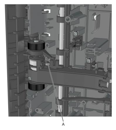
**9** Remove the other half of the cable from the printer.
