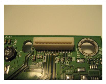
**2** Insert the cable squarely into the connector.
