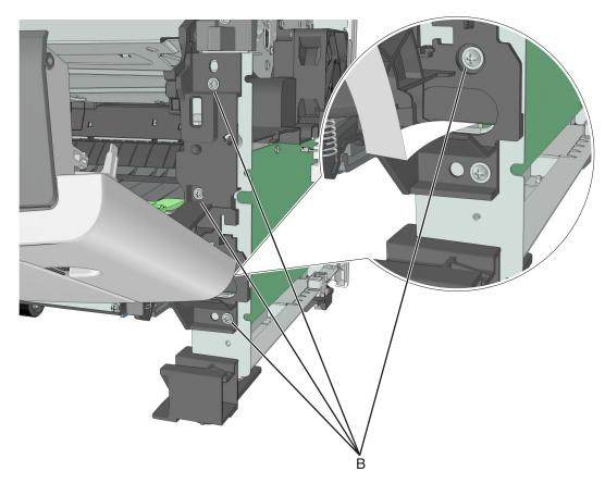
**7** Remove the right front mount, and then remove the front door. Below are the front door and the right front mount.
