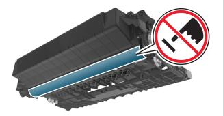
**4** Place the imaging unit aside on a flat, smooth surface.
