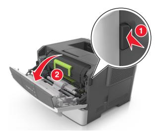
**2** Pull out the toner cartridge using the handle.
