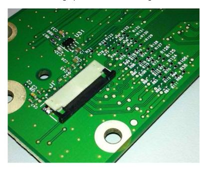
2 Insert the cable with the contacts on the cable facing away from the locking actuator. Insert the cable on top of the actuator.
