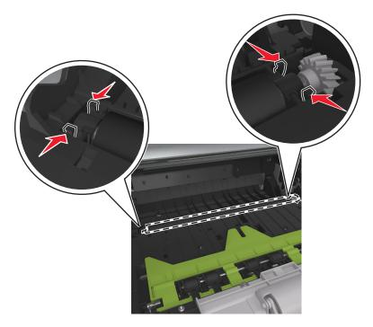
**2** Lift to remove the transfer roll.
