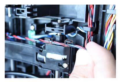
**d** Loop the cable behind the right cable holder.
