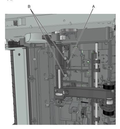
**9** Disconnect the cable from the sensor.
