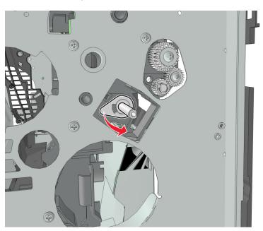
Pry the pointed end of the 2nd pickup pushing to release the locking pin underneath.
