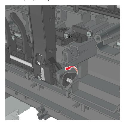
**14** Pull out the shaft, and remove the ACM.
