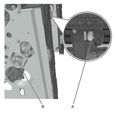
**6** Pull out the ACM clutch, and cut cable close to the clutch to detach it.
