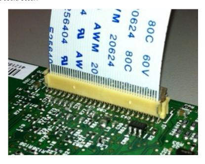
**3** Rotate the locking actuator to the locked position by pressing down on both ends of the actuator. The cable should not move when this step is performed. If the cable moves, open the actuator, reposition the cable, and then close the actuator to the down position.
