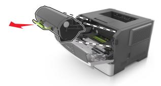
**3** Lift the green handle, and then pull out the imaging unit from the printer.
