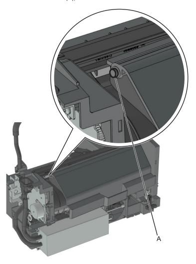
Using a flat-blade screwdriver, release the latches, then remove the input cover.
