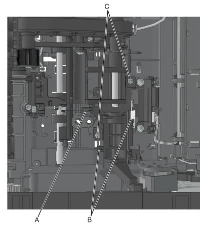
Below are the cam release and bracket.
