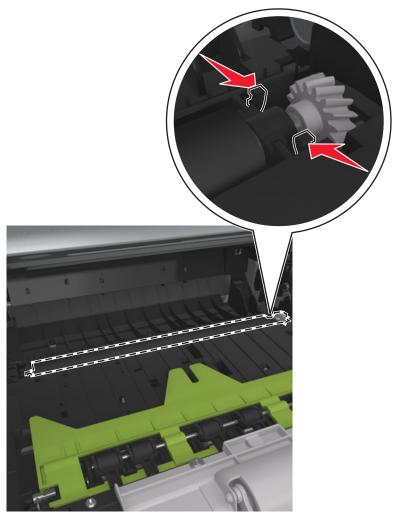
**2** Lift to remove the transfer roll.
