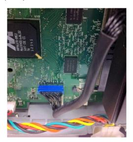
**4** Loosen the two screws (A) securing the modem to the controller board shield.
