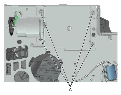
Disconnect the cable from the cartridge gearbox.
