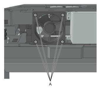
**7** Route the cable off the stapler, and remove the cooling fan.
