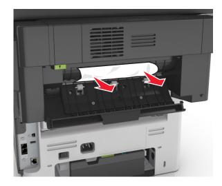
Open the finisher trap door, remove any paper fragments inside the trap door.
