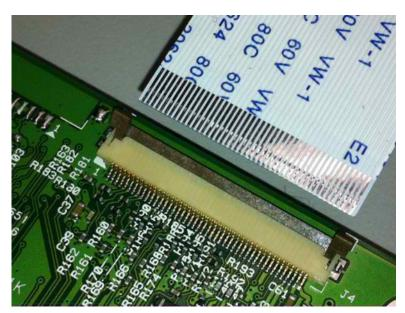
Rotate the locking actuator to the locked position. The cable should not move while this step is performed. If the cable moves, open the actuator, reposition the cable, and then close the actuator to the down position.
