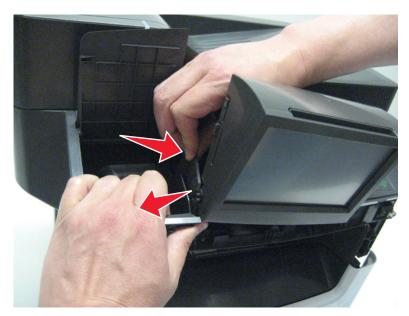
Remove the two screws (D) securing the toroid bracket to the control panel cover.
