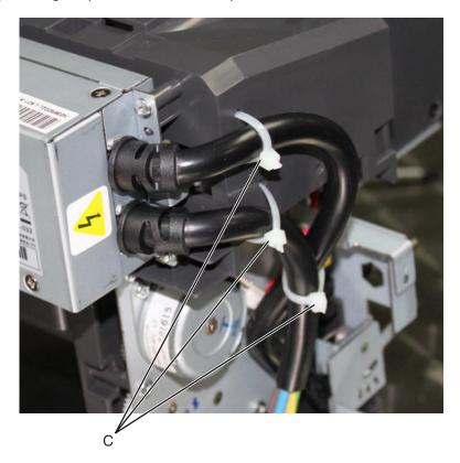
**10** Route the cable off the stapler, and remove the power supply unit.
