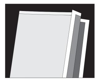
**4** If the grid lines of the right flap align below the corresponding lines on the left flap, then adjust the printhead clockwise relative to the printer, and recheck. If the grid lines of the left flap align below the corresponding lines of the right side, then adjust the printhead counterclockwise.
