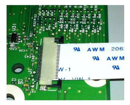
**3** Slide the locking actuator towards the connector, locking the cable into place. The cable should not move when this step is performed. If the cable moves, open the actuator, reposition the cable, and then close the actuator to the down position.
