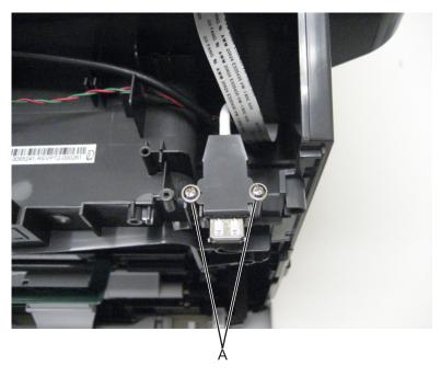
2 Remove the USB cable bracket.
