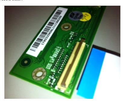
**3** Place your finger in the middle of the actuator, and then rotate the locking actuator to the locked position.
