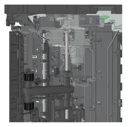
**c** Secure the cable near the lift plate gearbox using cable ties. Cut off any excess cable tie.
