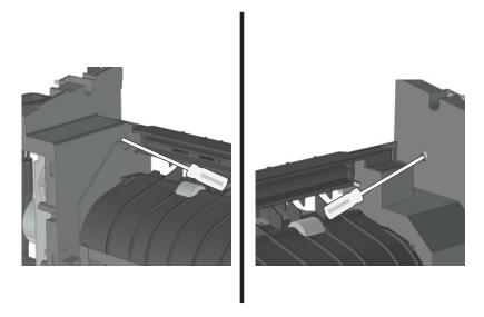
**5** Squeeze the latches to release, and dislodge the interface cable from its slot.
