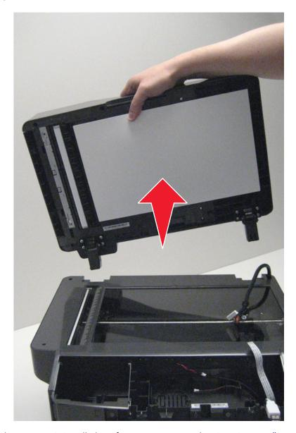
**Installation note:** After the new ADF is installed, perform scanner manual registration, see <u>"Scanner manual registration" on page 207</u> and scanner calibration, see <u>"Scanner calibration" on page 183</u>.
