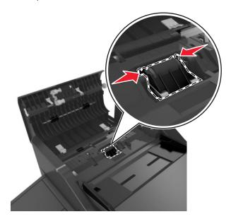
Pull away the separator roll and remove.
