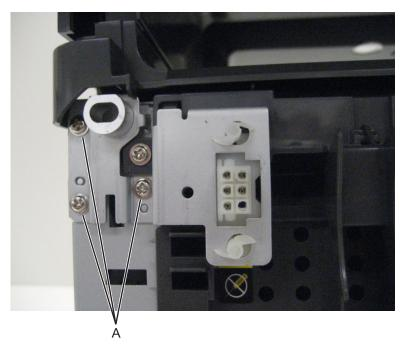
**6** Remove the stapler cable and mounting bracket from the printer frame while feeding the cable through the redrive unit and printer frame.
