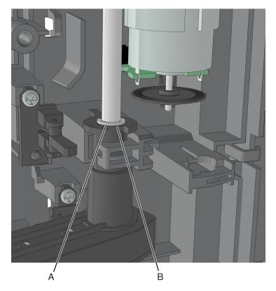
**8** Release the lock by sliding the bushing and then rotating it clockwise.
