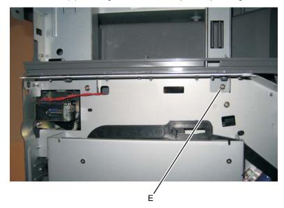
**19.** Remove the side screw (F) securing the right flatbed stop to the print engine frame.
