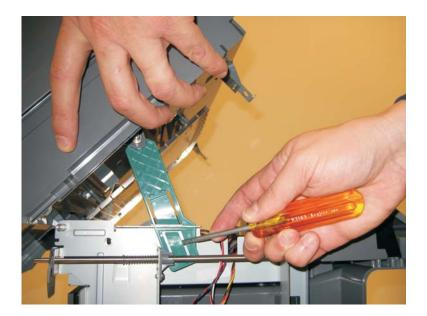
**10.** Remove the e-clip (A) from the flatbed hinge rod.
