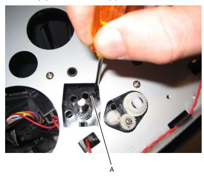
7. Use a small pair of pliers to remove the shaft retainer tab.
