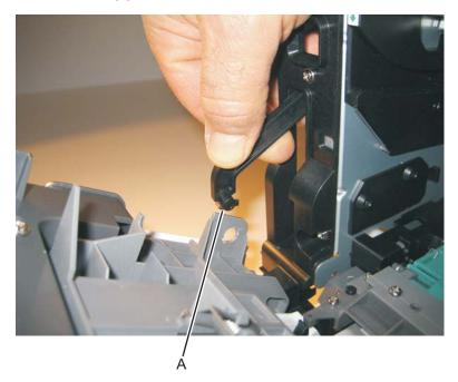
$\pmb{8.}\;\;$  Disconnect the front access door from its hinges, and remove.
