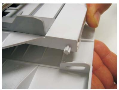
7. Open the front access door, and remove the lower paper guide.
