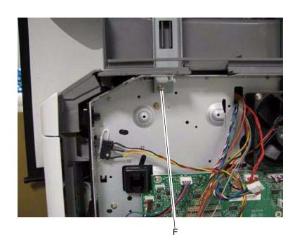
20. Lift and remove the scanner assembly from the MFP.
