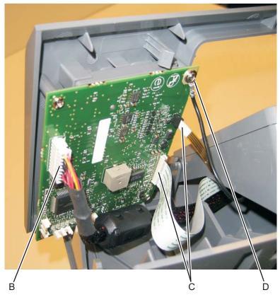
6. Tilt the operator panel keypad up and remove it from the MFP.
