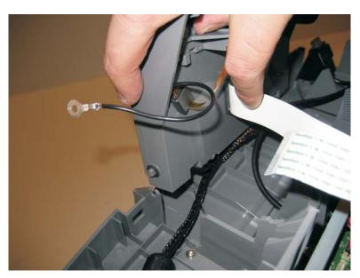
Note: Remove the operator panel display bezel from the old display. See "Display bezel" on page 3-64. It will be used on the new operator panel display.
