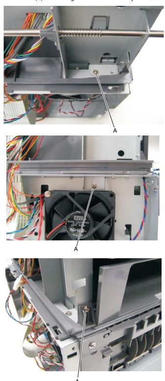
3. Carefully lift the right rear frame assembly off of the print engine frame.
