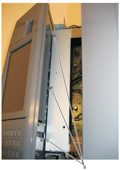
**3.** Loosen the three screws (C) on each side of the controller board cage.
