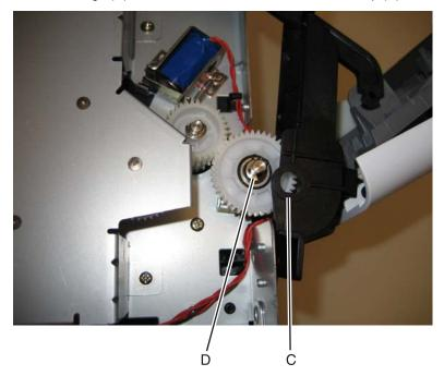
**7.** Lift and remove the multipurpose feeder (MPF) feed clutch.
