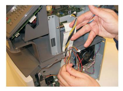
**12.** Disconnect LSU HSYNC extension cable at the connector in the middle of the cable.
