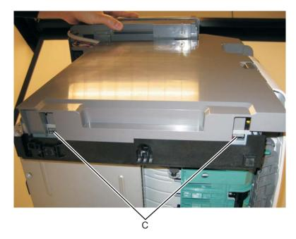
7. Lift the left cover up and pull the bottom of the cover away from the MFP.
