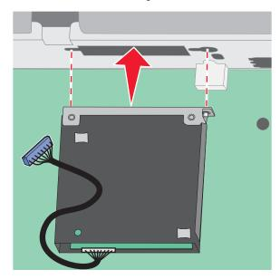
**5.** Tighten the two screws to secure it to the controller board cage.
