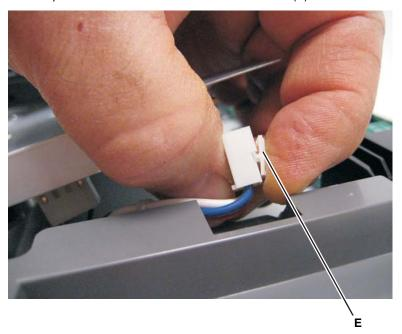
**8.** Disconnect the transfer roll cable (F).
