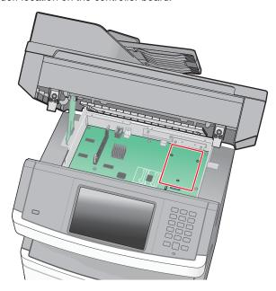
**Note:** If an optional printer hard disk is currently installed, then the printer hard disk must first be removed. See "Printer hard disk removal" on page 4-106.
