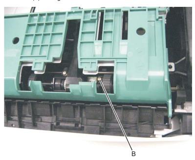
**6.** Free the cable from its retainers, and pull it through the opening toward the sensor mount.
