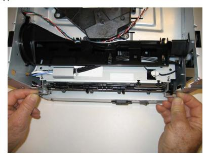
**4.** Push in on the cable connector cover (B), and remove.
