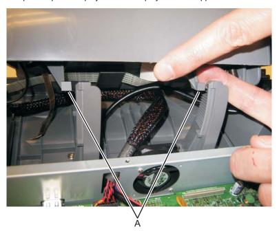
4. Disengage the operator panel display from the right display support and remove it from the MFP.
