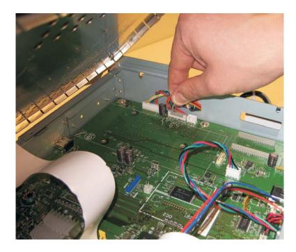
11. Thread the LSU diode cable, the cover interlock cable, the stairway cables, and the controller board power supply cable through the side of the printer away from the scanner assembly.
