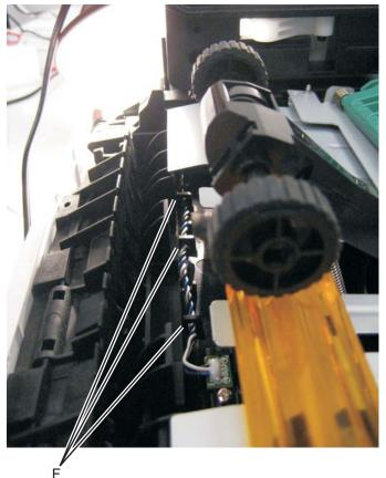
Note: If the cable is not properly installed in its retainers, then the loose cable will obstruct the paper path.
