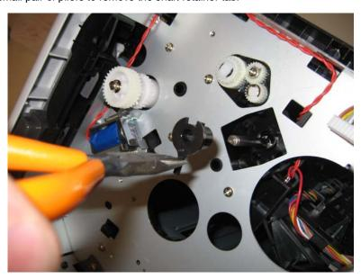
**8.** Use a screwdriver to pop the inner shaft lock (B) loose.
