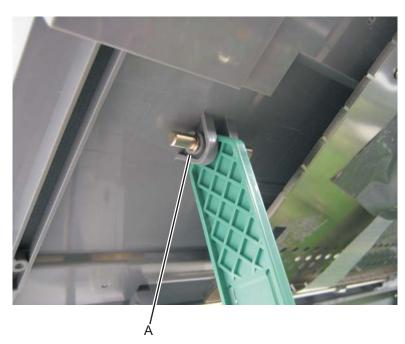
**4.** Slide the rod out and remove the kickstand from the flatbed.
