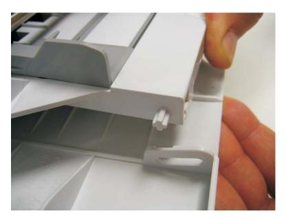
7. Disconnect the fuser link (A) from the front access door.
