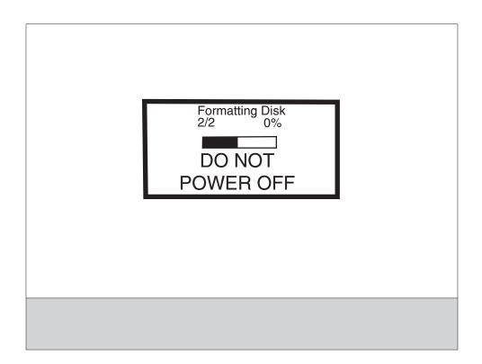
The entire process is complete when the progress bar appears completely shaded and the percentage indicator shows 100%. After completion, the panel returns to Disk Encryption.
