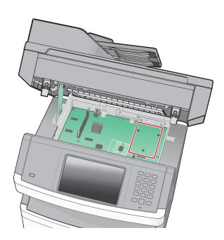
**4.** Use a flatblade screwdriver to remove the screws attaching the mounting bracket.
