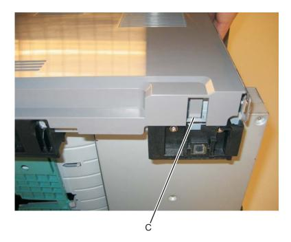
**5.** Rotate the right side cover assembly slightly to the left, and pull out.
