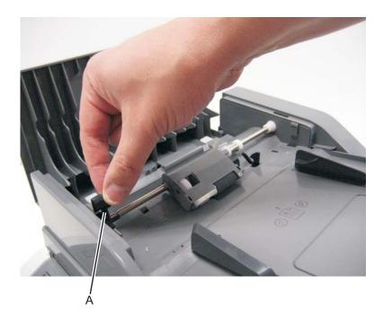
2. Slightly lift the separator roll assembly, and pull it out of the mount (B) on the opposite side.
