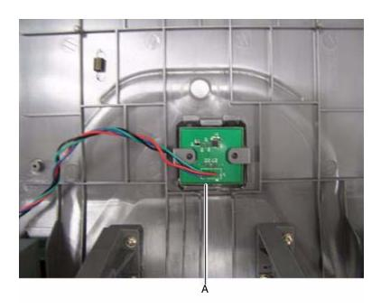
4. Pull down on the lens and LED and remove it from the tub.
