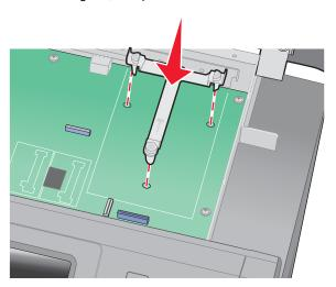
6. Install the ISP onto the plastic tee.
