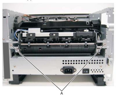
**3.** Partially pull the fuser forward for better access.
