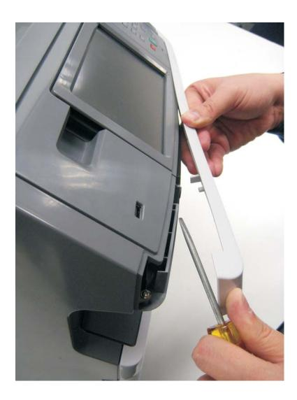
**2.** Carefully pull the scanner front cover away from the tub assembly.
