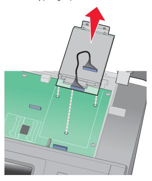
4. Remove the thumbscrews that attach the printer hard disk mounting bracket to the printer hard disk if the drive is going to be installed on top of an ISP.
