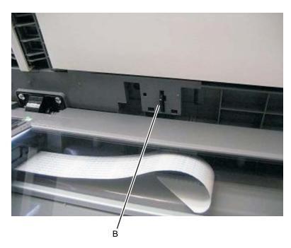
5. To test scanner sensor 1 press on the tab (C). The 0 next to the 1 will change to 1 if the sensor is working properly.
