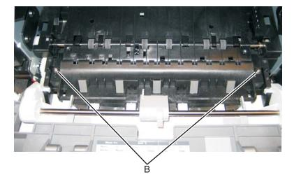
**5.** Close the front access door, and pull up on the MPF by the steel shaft until the MPF lifts from its hinges.
