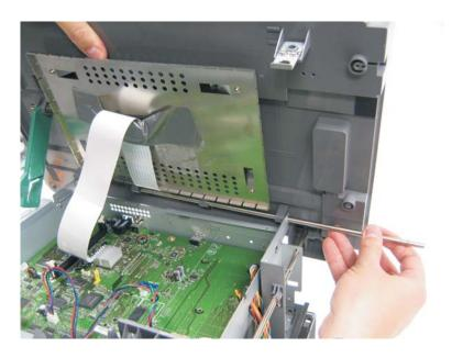
12. Lift and remove the flatbed unit from the MFP.
