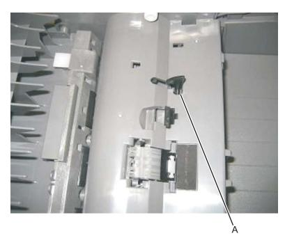
4. To test the flatbed cover closed sensor, lift the flatbed cover. The 0 next to the F will change to 1. Also check the actuator (B) to ensure it is functiong properly.
