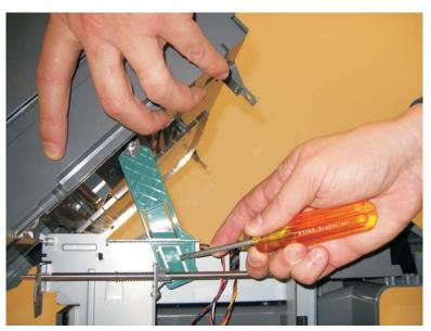
**3.** Remove the e-clip (A) securing the kickstand rod to the flatbed.
