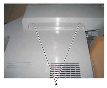
**3.** Lift and carefully pull the right scanner cover up and away from the rear of the flatbed.
