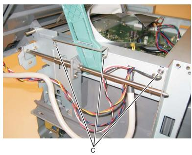
**4.** Remove the controller board shield.
