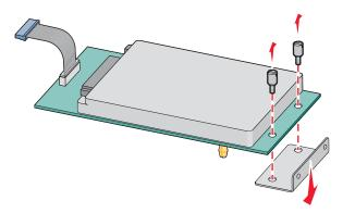
**5.** Place the hard disk on top of the ISP, making sure the standoff on the hard drive line up with the holes on the ISP.
