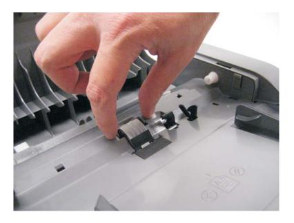
**3.** Tilt the pad up, and lift it out of the ADF assembly.
