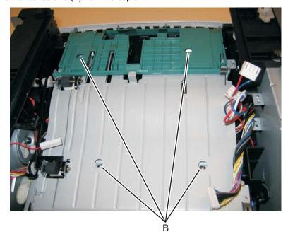
**5.** Lift the duplex slightly, push to the left, and tilt to clear the right side of the printer.
