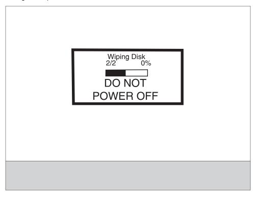
The entire process is complete when the progress bar appears completely shaded and the percentage indicator shows 100%. The panel returns to the screen that shows the values for the Wipe Disk setting.
