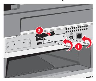
**4.** Insert the fax card into the controller board cage.
