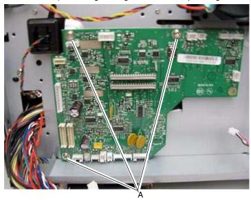
**4.** Remove the engine board.
