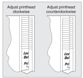
**8.** After obtaining a properly adjusted image on the paper, tighten all three screws.
