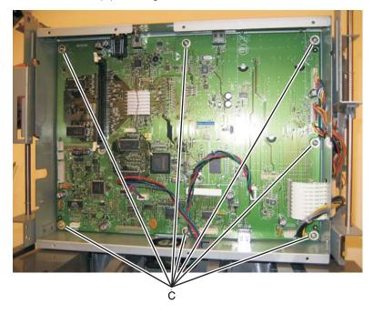
**12.** Lift the controller board, and remove.
