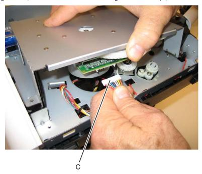
**6.** Remove the main motor gear drive.
