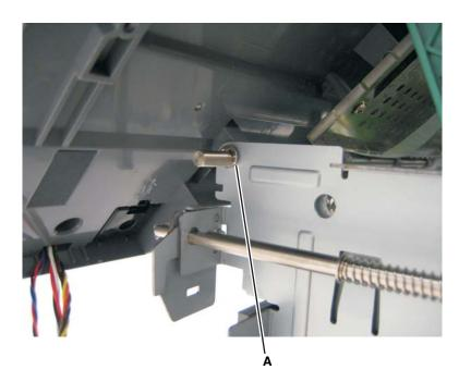
**11.** While holding the front of the flatbed with one hand, pull the flatbed hinge rod out.
