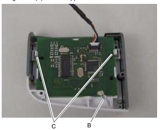
7. Pull the two tabs (C) back and remove the card from the card reader housing. Note: When replacing the light tube, cover the tube with a small piece of black electrical tape if possible.
