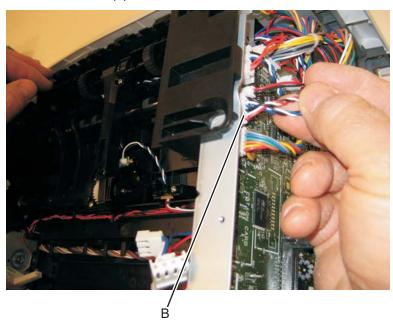
5. Remove the paper input and duplex sensor assembly.
