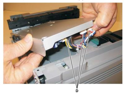
Note: Squeeze the clip to remove the cables from their connectors (E).
