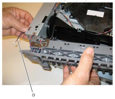
7. Remove the rear exit guide assembly.
