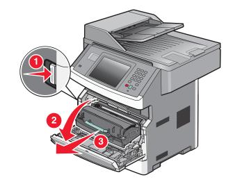
2. Lift the flap at the front of the MFP, and remove any jams.
