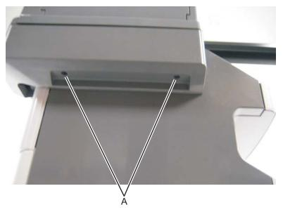
**3.** Lift and carefully pull the left scanner cover up and away from the rear of the flatbed.
