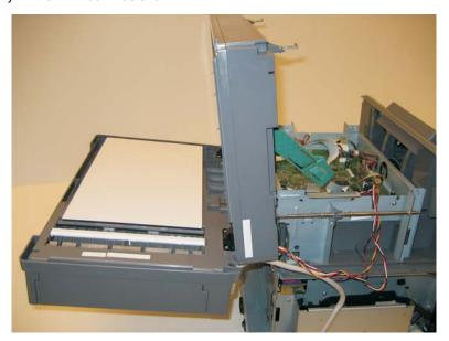
Warning: To avoid damage to the rear frame assemblies, hold the ADF while raising the flatbed to the upright position, then lower the ADF, slowly a shown above.
