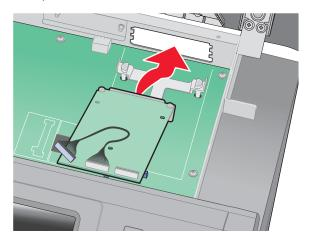
**Note:** Make sure the ISP card is properly aligned with the rear of the controller board cage.
