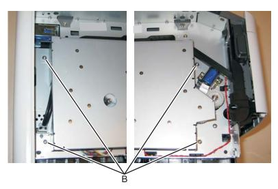
**5.** Rotate the main motor gear drive enough to access the manual feed solenoid.
