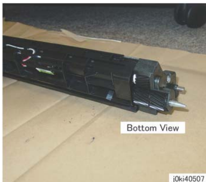
Figure 16 Check/clean Developer Housing Assembly gears
