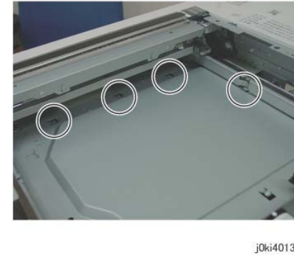
Figure 9 Install the PWB Cover
