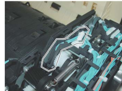
Figure 6 Remove the disconnected wire harness
