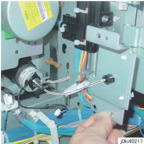
Figure 4 Installing the Bracket
