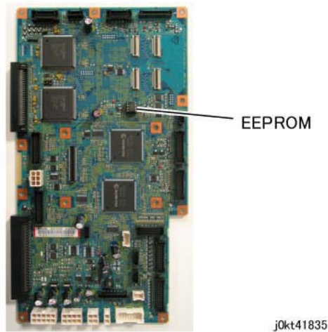
Figure 7 Remove the EEPROM
