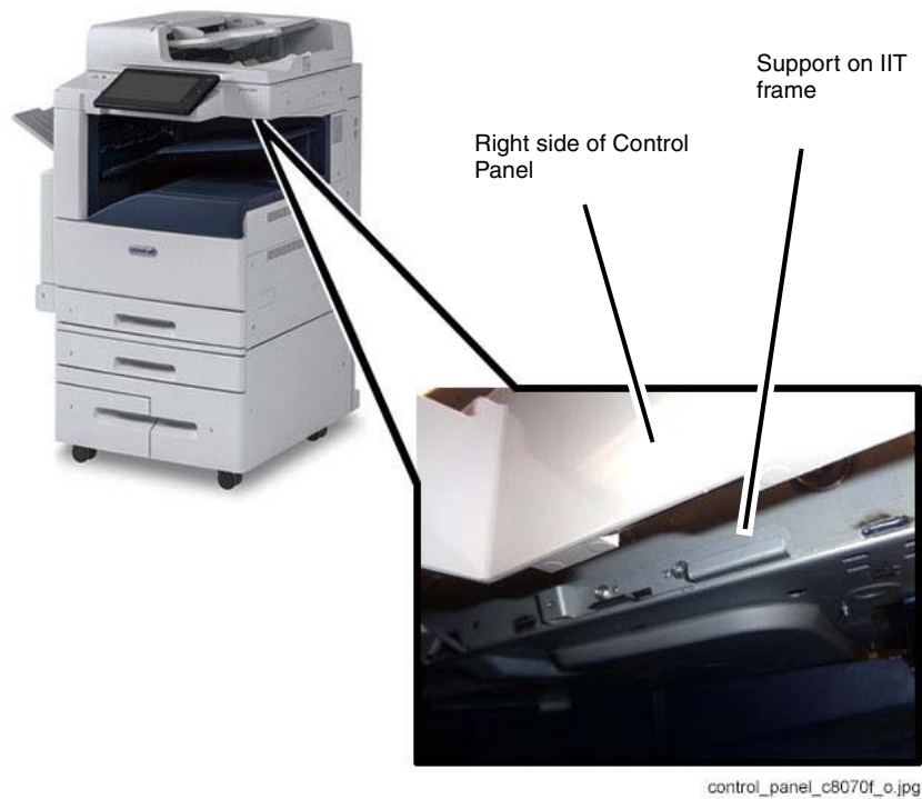
Figure 6 Removing the Control Panel
