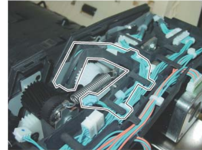
Figure 5 Remove the disconnected wire harness
