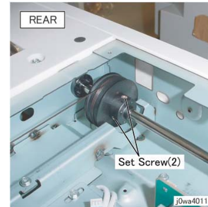
Figure 3 Loosen the rear pulley
