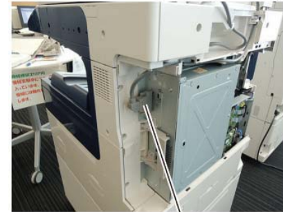
Figure 1 Disconnect the Connector
