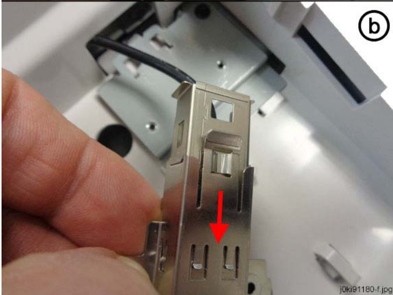
Figure 4 Slide off the USB B ratchet
