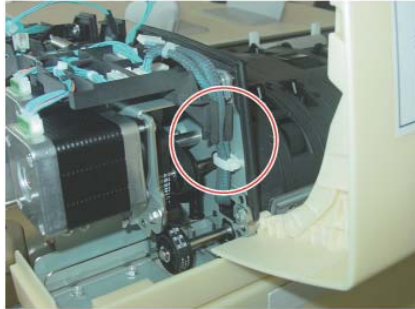
Figure 7 Remove the disconnected wire harness
