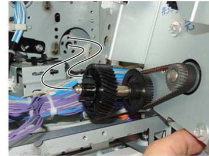
Figure 29 Install the gear and shaft
