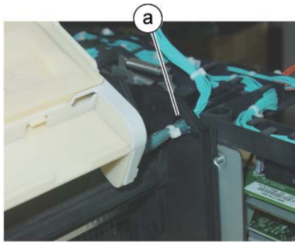
Figure 4 Remove the wire harness
