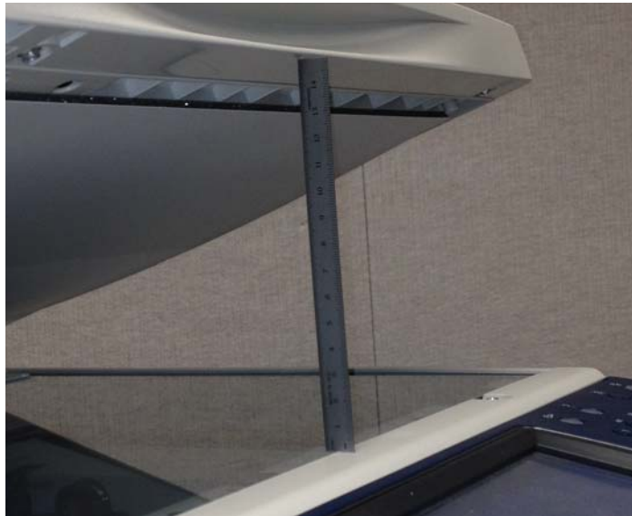
Figure 1 Open the DADF 150mm (5.9 in)
