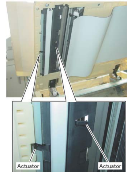
Figure 4 Check the actuators
