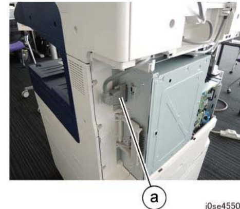
Figure 1 Disconnect the connector
