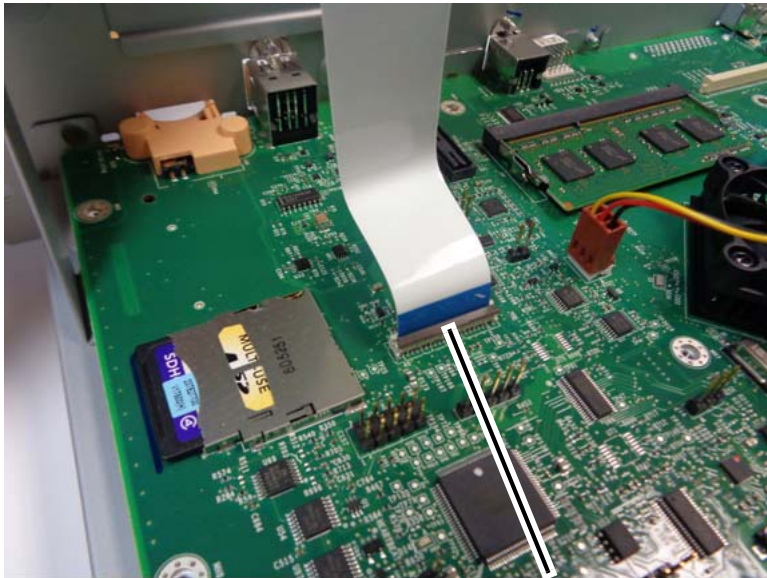
1 Lift the tab and remove cable
