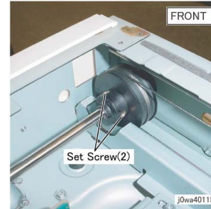
Figure 2 Tighten the front pulley
