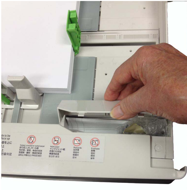
Figure 1 Tray 1 Storage Compartment
