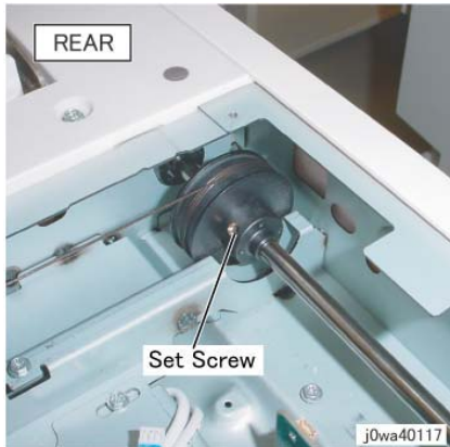
Figure 5 Tighten one of the set screws
