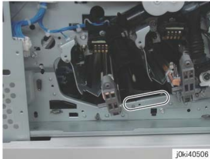
Figure 15 Check/clean before installing the Developer Housing Assembly
