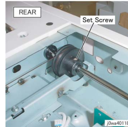
Figure 7 Tighten the set screw
