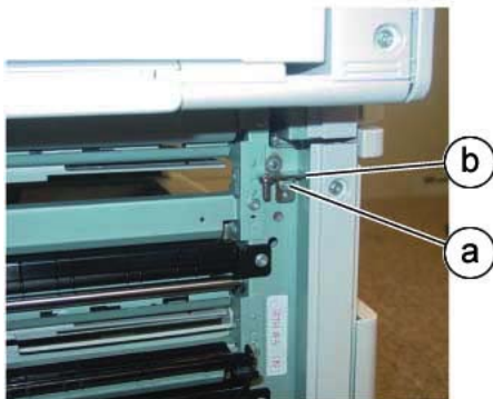
Figure 2 Removing the Bracket Assembly
