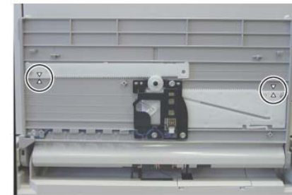
Figure 5 Installing the Pinion Gear
