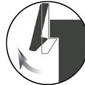
Figure 2 Plastic latch release
