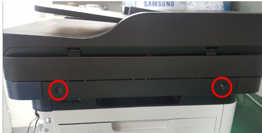
Figure 1 Scanner screw removal
