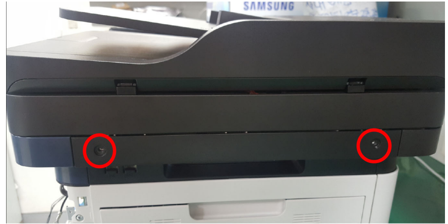
Figure 1 ADF / Scanner screws removal
