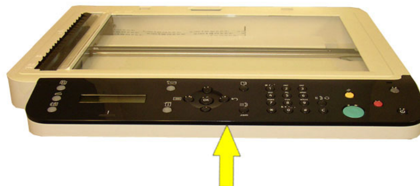
Figure 2 Control Panel release
