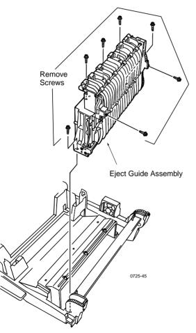
Removing the eject guide assembly
