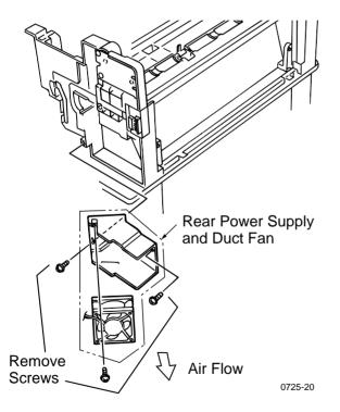
Removing the rear power supply fan
