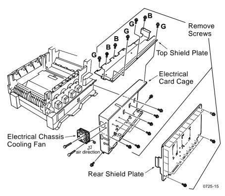
Removing the electrical card cage
