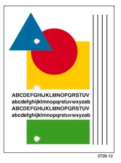
94 mm (3.7 in.): Imaging drum. Replace the imaging drum unit.
