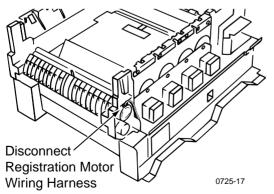
Disconnecting the registration motor in-line connector (HOPFF)
