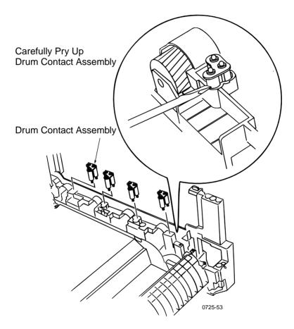
Removing the drum contact assembly
