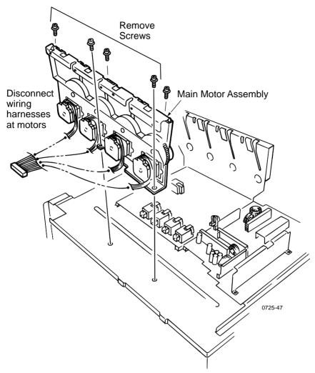
Removing the main motor assembly
