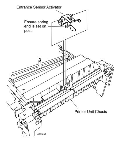
Removing the tray 1 entrance sensor actuator
