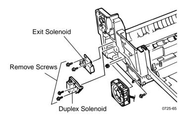
Removing the duplex solenoid and the exit solenoid
