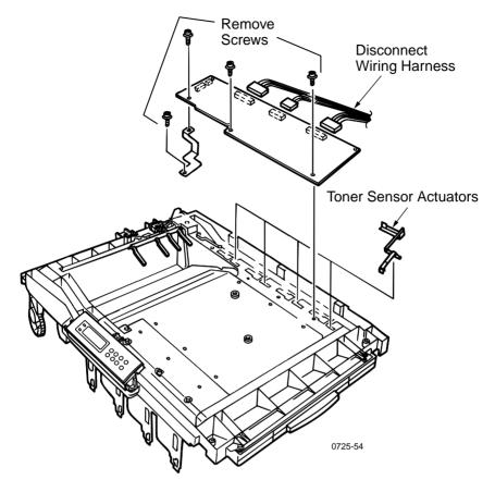
Removing the toner sensor actuators
