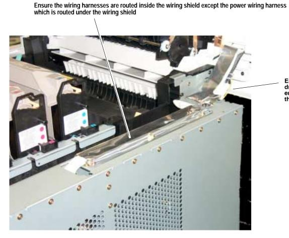
Ensure the power harness inter-connect is dressed behind the flat ribbon cables to ensure it does not disconnect when the top cover is closed
