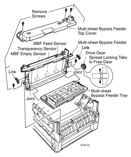
Removing the multi-sheet bypass feeder
