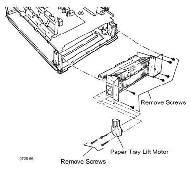
Removing the main feeder assembly
