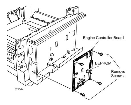
Removing the print engine controller
