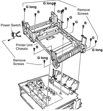
Removing the printer unit chassis
