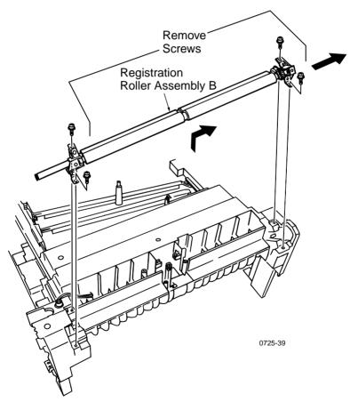
Removing the registration roller assembly B
