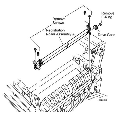
Removing the registration roller assembly A and drive gear
