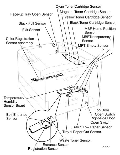
Print engine sensor and switch locations
