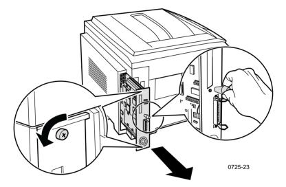
Removing the system controller board
