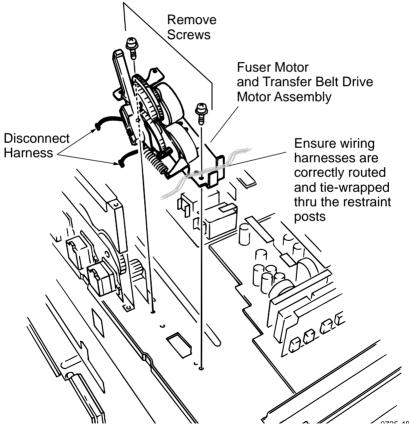
Removing the fuser motor and transfer belt drive motor assembly
