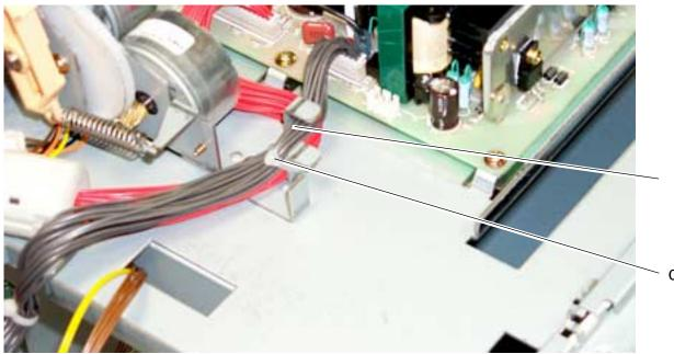
Route wiring harnesses between first and second restraint posts
