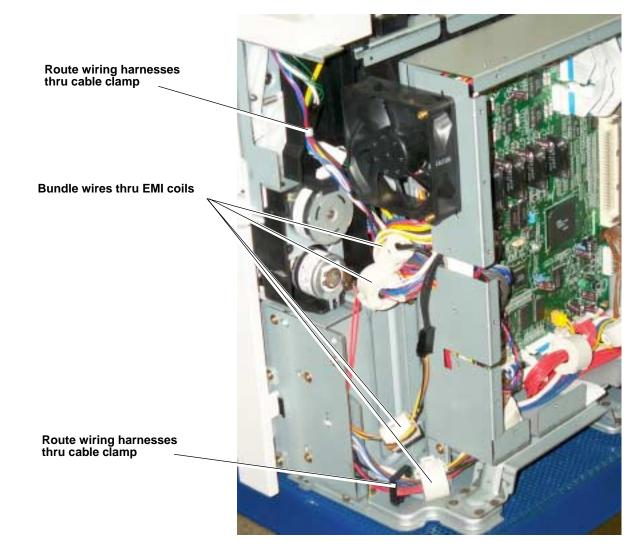
Details of wiring passthru
