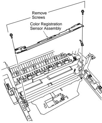
Removing the color registration sensor assembly
