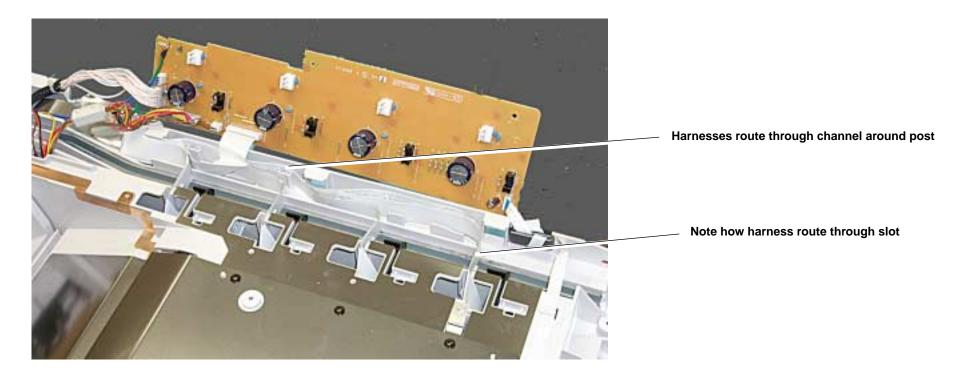
Ribbon cable routing under the toner sensor board
