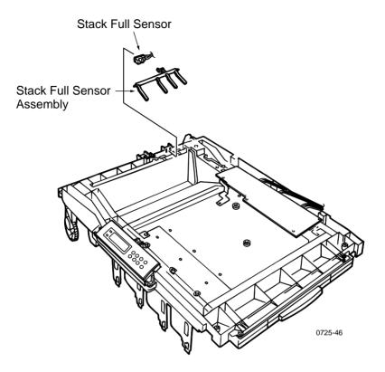
Removing the stack full sensor
