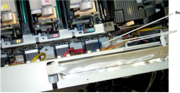
Route wiring harnesses under the imaging drum motors
