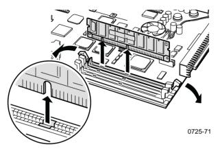
Removing the RAM DIMMs
