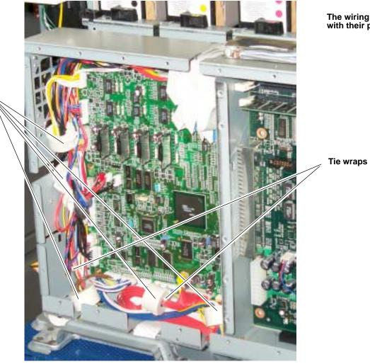
Bundle wires thru EMI coils
