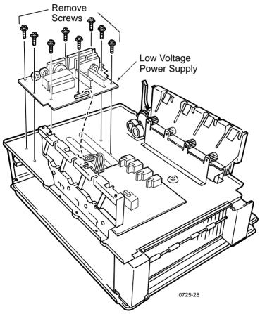
Removing the low voltage power supply
