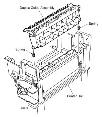
Removing the duplex guide assembly
