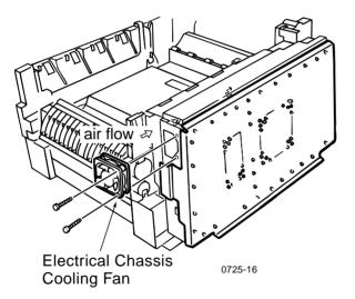
Removing the electrical card cage cooling fan
