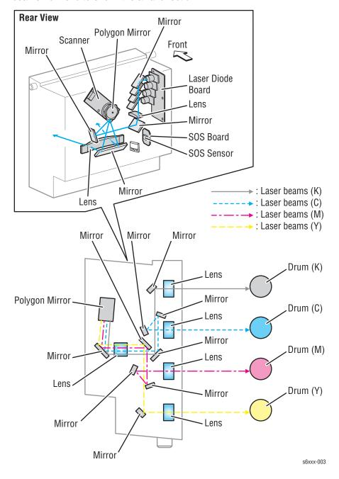
The negatively charged Drum surface is scanned by the laser beams to form an invisible electrostatic latent image on the drum surface. The process is performed in parallel for Cyan, Magenta, Yellow, and Black colors.
