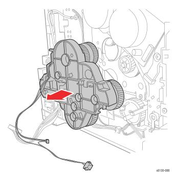
7. Unplug the color mode sensor connector (P/J261) from the Feed Drive Assembly and release the Color Mode Sensor Harness from the hook on the Feed Drive Assembly.
