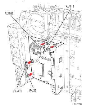
4. Remove 4 screws (silver, 6mm) that attach the Image Processor Board and the I/O Plate to the printer, and remove the Image Processor Board from the printer together with the I/O Plate.
