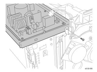
14. Release the hook of the connector of the RL Test Harness using a pliers, and then remove it from the Dispenser Assembly.
