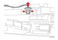
**15.** Remove the Fuser Harness, LVPS Harness, 24V Harness, I/P Board Power Harness and Harness B from the hooks on the Dispenser Assembly.
