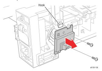
5. Pull the GFI Breaker out of the frame, unplug the three connectors (P/ J482, 483, 484), and remove the GFI Breaker from the printer.
