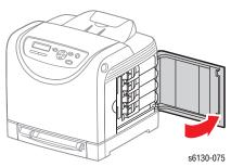
2. Press down on the upper hinge of the Toner Access Door to release the boss on the hinge from the hole in the Right Side Cover, and tilt the Toner Access Door down so that its top hinge clears the printer frame.
