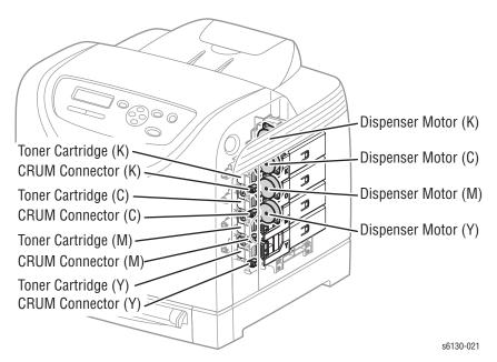
The Toner Cartridge is a customer replaceable item that includes the following components:
