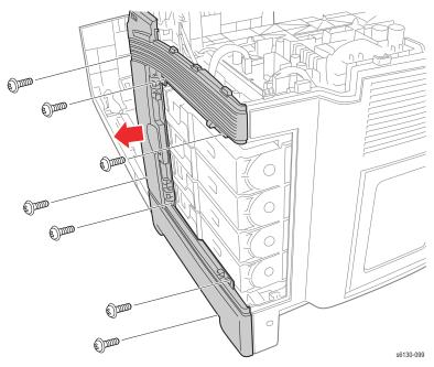
5. Release the hook at the front and remove the Right Side Cover from the printer.
