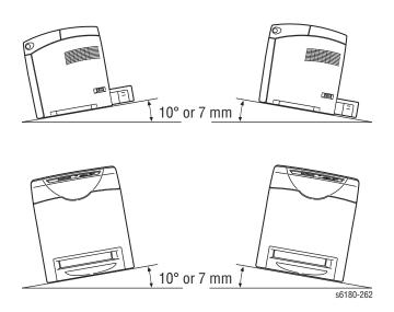
Failure to adhere to the specified mounting specifications will void all guarantees of print-quality and/or performance. Known problems that can occur as a result of exceeding the mounting surface specifications are:
