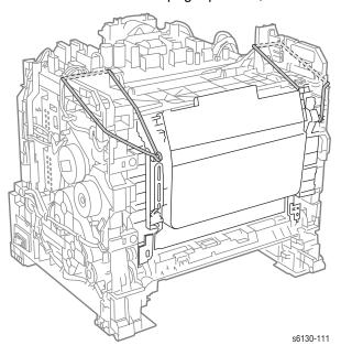
4. Disconnect the plug (P/J281) on the Transfer Unit, then remove the cover from the harness guide, and release the harness wires from the guide.
