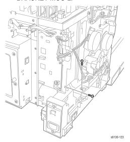
18. Lift the Upper Assembly off of the Lower Assembly.
