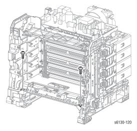
13. Remove the screw (silver, tap, 8mm) that attaches the right Transfer Unit Pivot Shaft to the Lower Assembly, but do not remove the Pivot Shaft.
