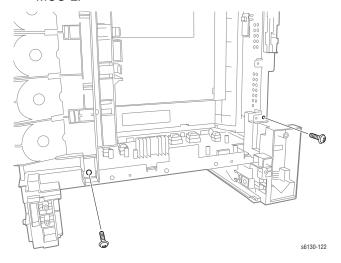
17. Remove the screw (silver, tap, 8mm) that attaches the left side of the printer frame and the screw (silver, tap, 8mm) that attaches the BRACKET MCU L.
