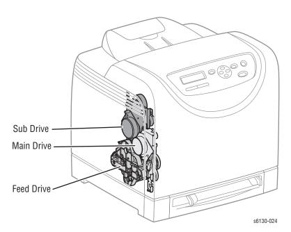
The Drive Assembly consists of three major sections:
