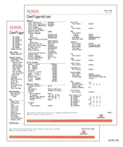
User can print the Configuration Page from the Control Panel > Menu > Information Pages > Configuration. The Configuration Page is printed in from the default tray and includes the following information.
