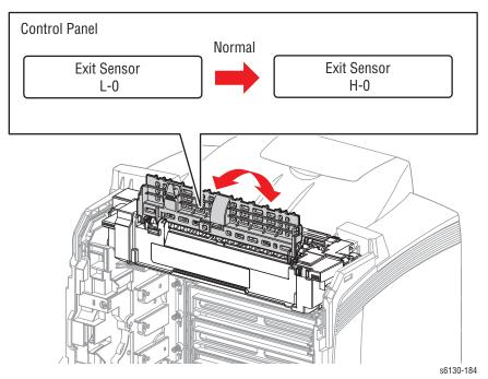
5. Press the **Cancel** button to stop the Exit Sensor test.
