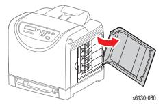
3. Lift the Toner Access Door up and out to remove it from the printer.
