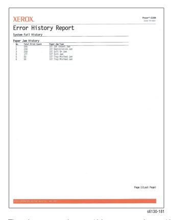
The printer can retain up to 42 jam errors and up to 42 fatal errors. User can print the Error History Report default on A paper size from default tray using the printer menu in the Control Panel.
