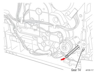
Remove the screw (silver, tap, 8mm) that attaches the Right Side Pivot Shaft to the printer.
