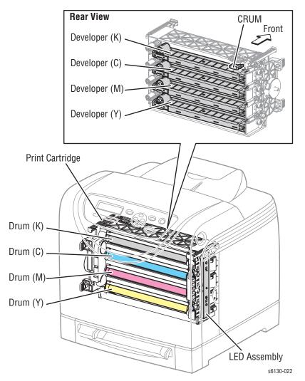
The Imaging Unit is a customer replaceable item that carries out the charging, development, transfer, and cleaning steps in the print process (see "Printing Process" on page 2-3).
