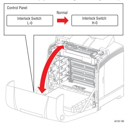
6. Press the Cancel button to stop the Cover Open Sensor test.
