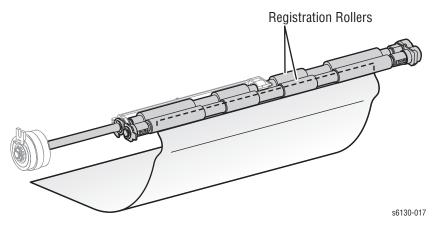
Before the Registration rollers are energized, the paper is advanced from the tray to the rollers. This process aligns the leading edge as shown below.
