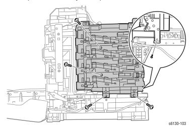
**18.** Release the hole in the Dispenser Assembly from the boss on the printer. Move the Dispenser Assembly toward the rear to remove it from the printer.
