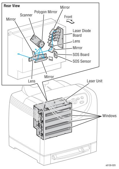
The Laser Unit is an exposure unit that generates laser beams to form an electrostatic latent image on the drum surface. The Laser Unit consists of the following components: Laser Diode (LD) Board, Scanner Assembly, Start of Scan (SOS) Board, Lenses, Mirrors, and Windows.
