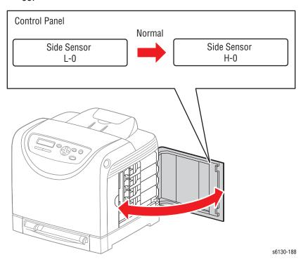
4. Press the Cancel button to stop the Side Switch test.
