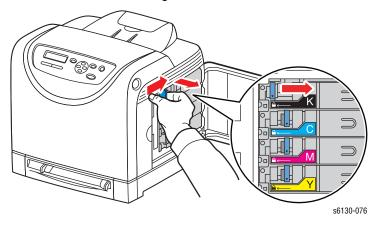
**3.** Swing open the toner cartridge holder and slide the toner cartridge out of the holder as shown.
