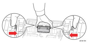
3. Pull the Separator Roller up to remove it from the Tray.
