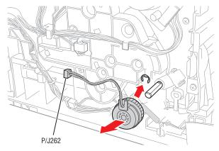
5. Release the two hooks of the Registration Bearing, and remove the Registration Bearing from the shaft.
