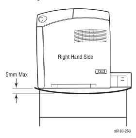
2. The printer must not be tipped or tilted more than 7 mm.
