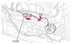
4. Remove the E-ring that secures the Drive Clutch on the shaft, using a miniature screwdriver, and remove the Drive Clutch.
