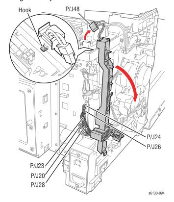
11. Remove the screw (silver, machine, 6mm) that attaches bottom of the Right MCU Bracket to the HVPS bracket.
