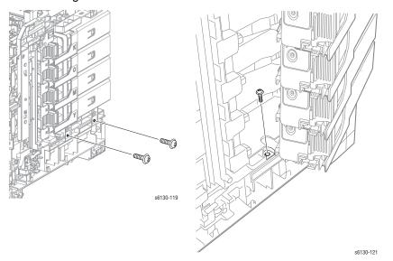
**16.** Remove the screw (silver, 6mm) that attaches the rear side of the Dispenser Assembly and the screw (silver, tap, 8mm) that attaches the MCU L.
