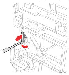
5. Rotate the Imaging Unit Lever slightly and remove it from the printer.
