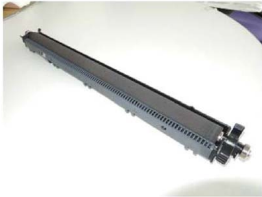
Figure 2 Removed BTR roll
