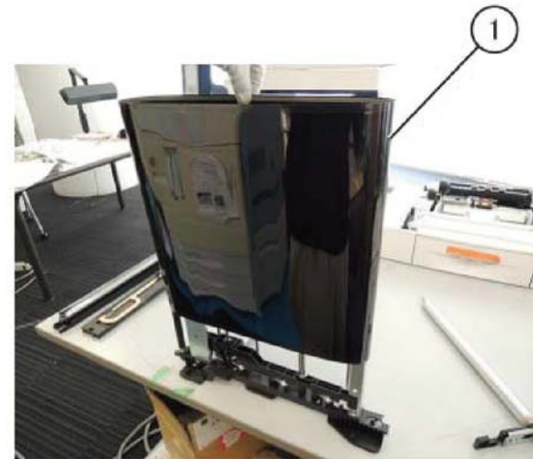
Figure 12 IBT belt unit replacement
