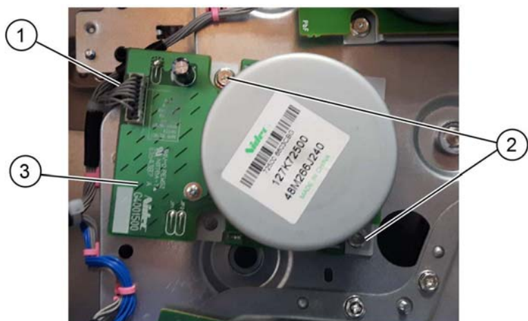
Figure 1 Main motor PWB removal
