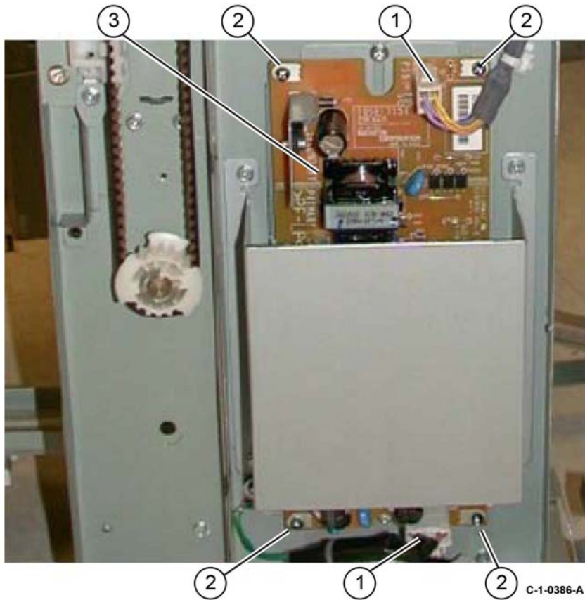
Figure 1 Finisher LVPS removal
