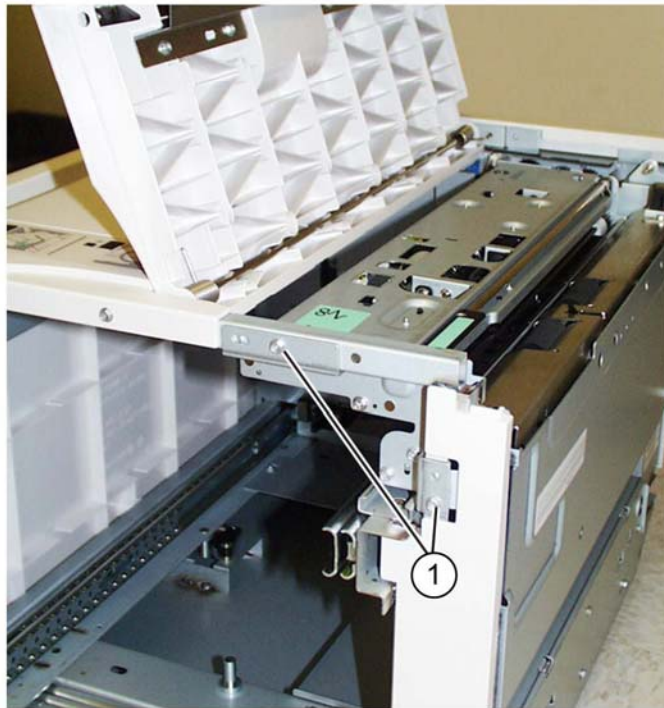
Figure 1 Feeder securing screws
