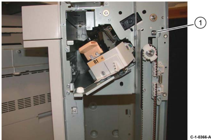
Figure 5 Front E-ring removal
