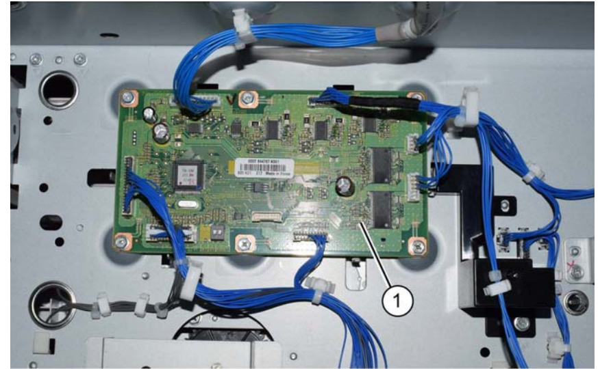
Figure 2 TTM PWB removal
