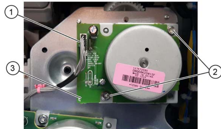
Figure 1 Fusing unit drive removal
