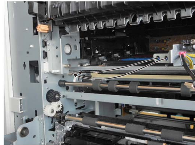
Figure 4 MOB ADC assembly install
