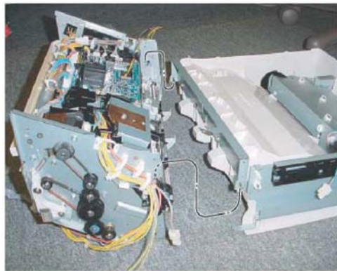
Figure 5 Stacker tray assembly installation
