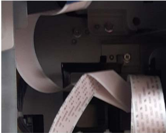
Figure 6 FFC guide removal
