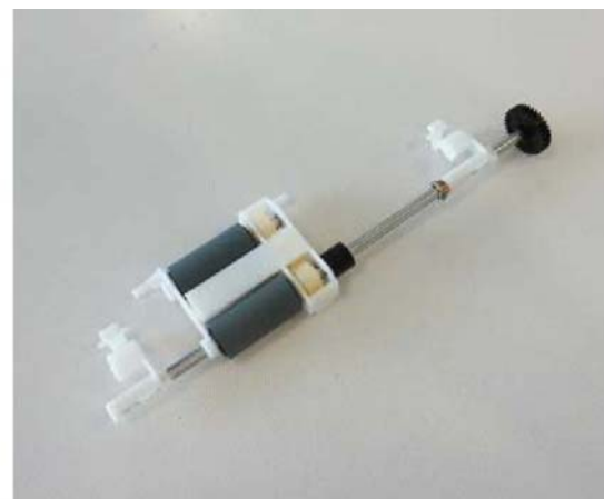
Figure 2 Removed feed/nudger roll assembly
