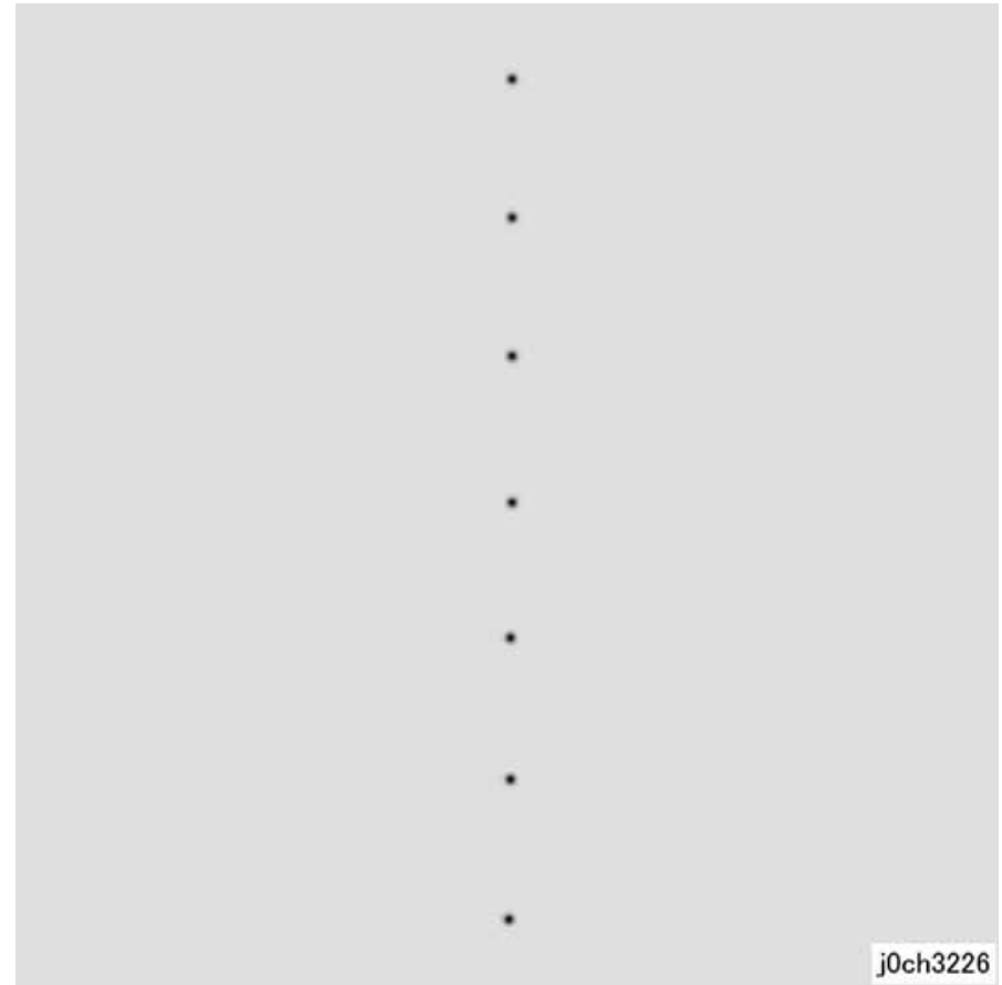
Figure 1 Regular Toner Contamination In Process Direction (Spots, Streaks, Bands etc.) Defect Sample (j0ch3226)
