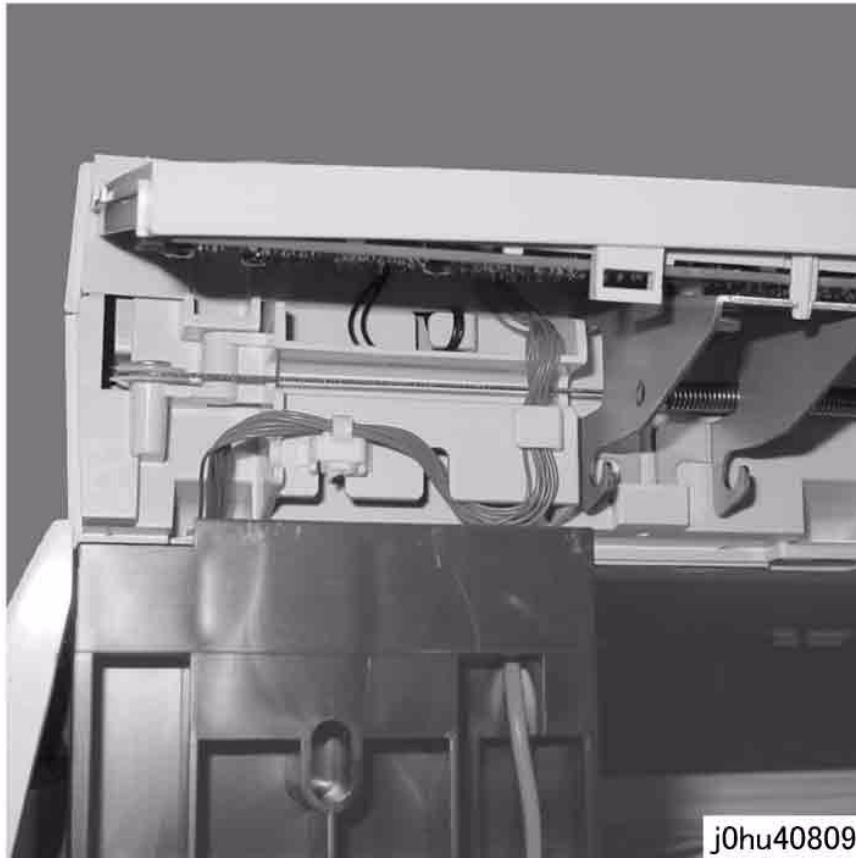
Figure 5 Threading Control Panel Harness
