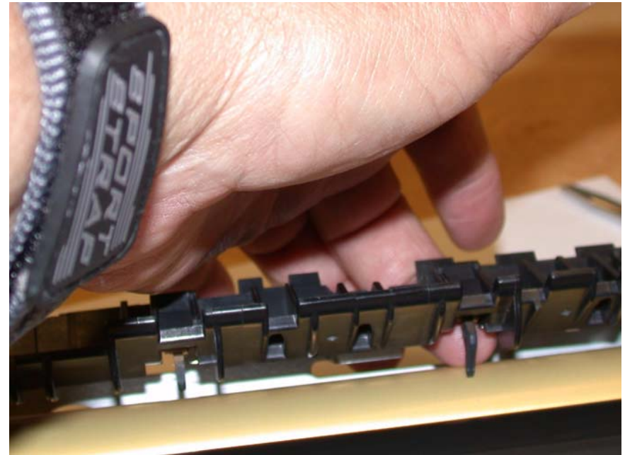
Figure 7 Setting the Stripper Fingers
