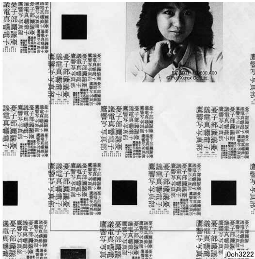
Figure 1 Toner Splattering Defect Sample (j0ch3222)
