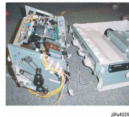
Figure 5 Installing the Stacker Tray Assembly (j0fa42251)
