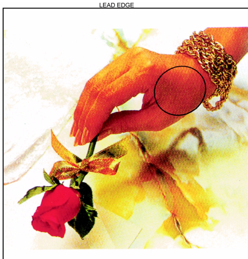
Figure 1 Moire Defect Sample
