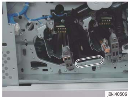
Figure 14 Check/clean before Installing the Dev.eloper Housing Assembly
