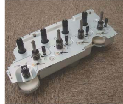
Figure 6 Place the Motor section facing downwards
