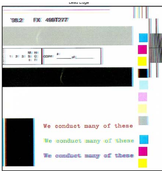
Figure 1 Color Misregistration Defect Sample
