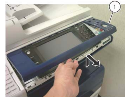
Figure 5 Remove the Overlay Cover
