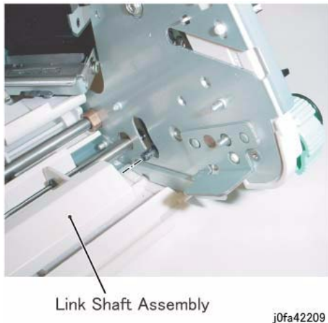
Figure 9 Installing the Paddle Link Assembly
