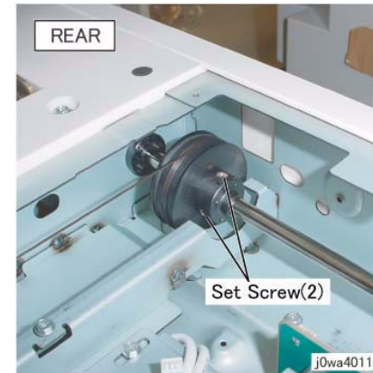
Figure 3 Loosen the rear Pulley
