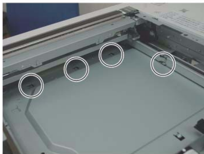
Figure 9 Install the PWB Cover
