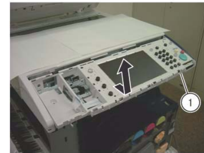
Figure 9 Moving the Console Assembly in the direction of the arrow
