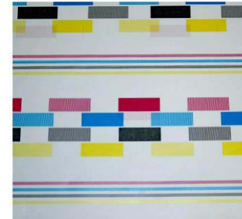
Figure 1 Video Data/Crosstalk Defect Sample
