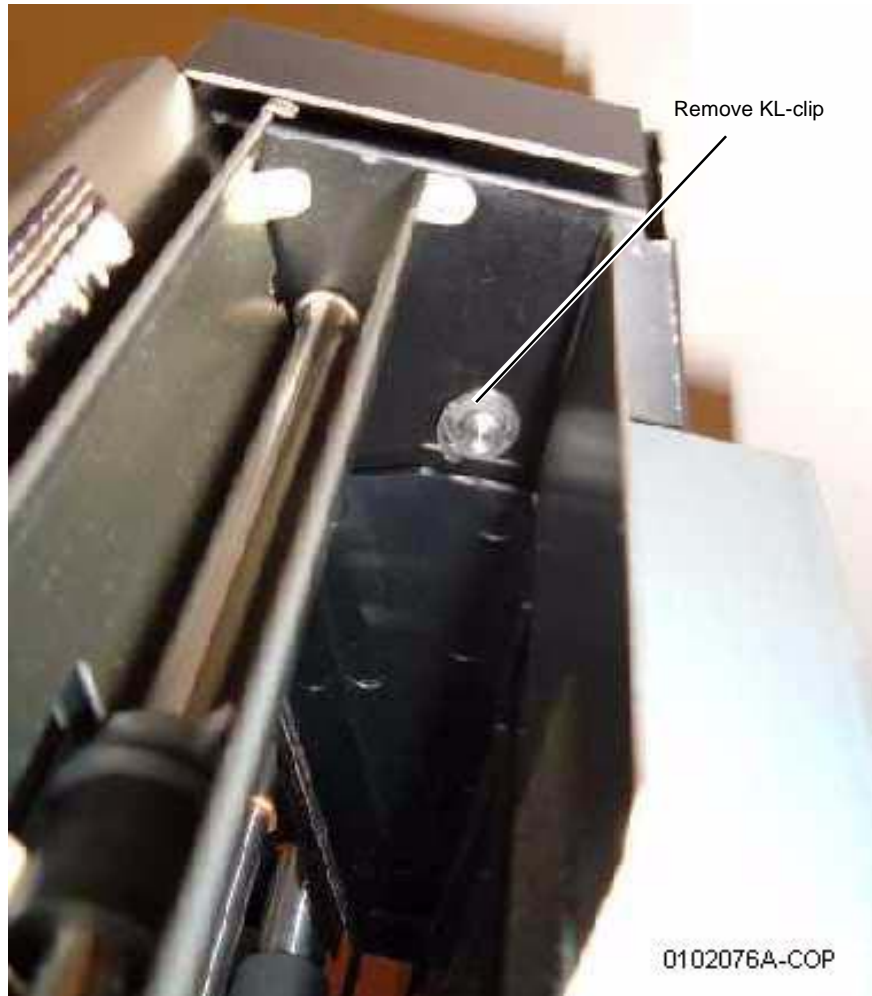
Figure 1 Removing the KL-clip
