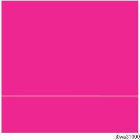
Figure 1 1mm Lines Defect Sample
