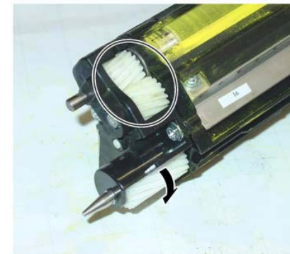
Figure 11 Make sure that no Dev.eloper or toner is stuck to the gears
