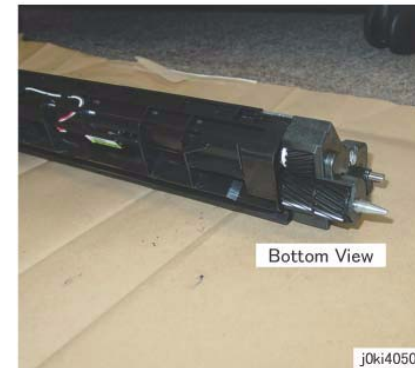
Figure 15 Check/clean Dev.eloper Housing Assembly gears
