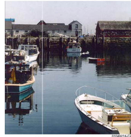
Figure 1 Streak Deletion Defect Sample
