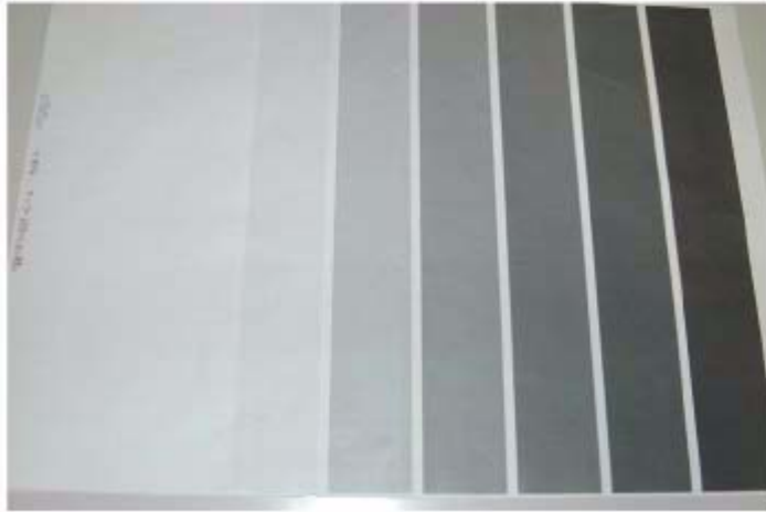
Figure 1 Tapes Not Peeled Defect Sample
