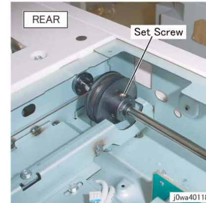
Figure 7 Tighten the set screw
