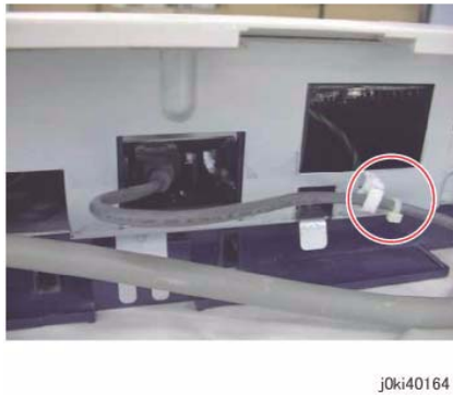
Figure 5 Align the cable
