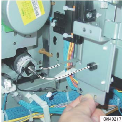
Figure 10 Install the Bracket
