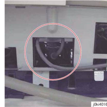
Figure 6 Push in the excess length of USB Cable
