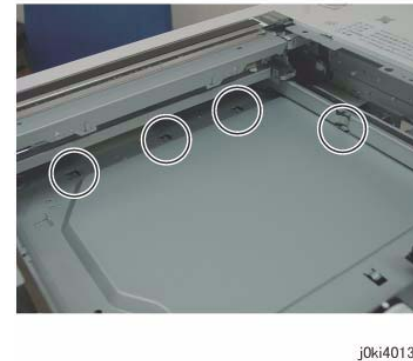
Figure 7 Install the PWB Cover
