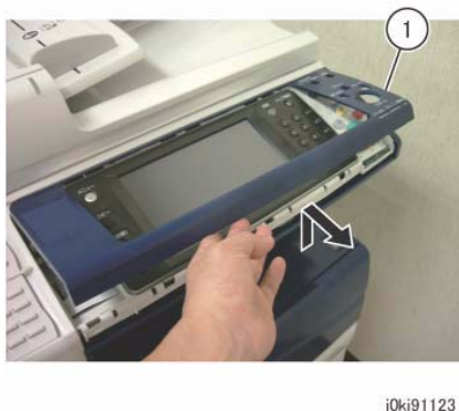
Figure 2 Remove the Overlay Cover
