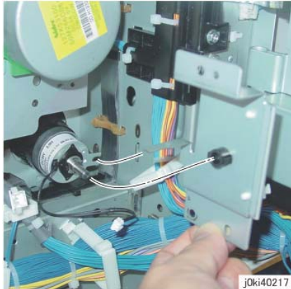
Figure 4 Install the Bracket
