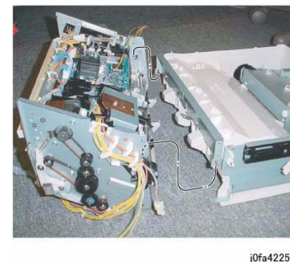
Figure 5 Installing the Stacker Tray Assembly
