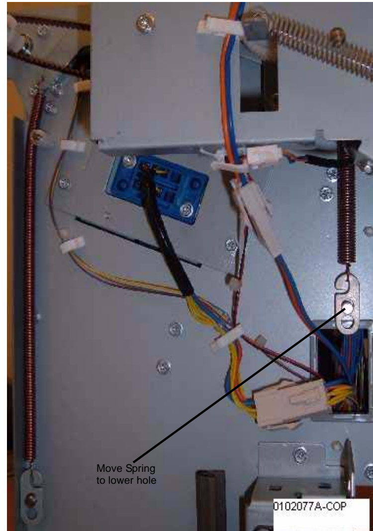
Figure 4 Adjusting the rear Spring tension
