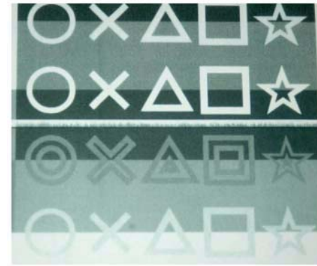
Figure 1 SLED Transfer Failure Defect Sample
