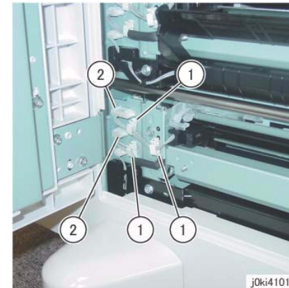
Figure 3 Disconnect the connectors
