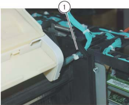
Figure 4 Remove the wire harness
