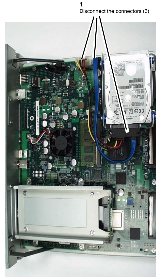
Figure 1 Disconnecting the Disk Drive Connectors (3)
