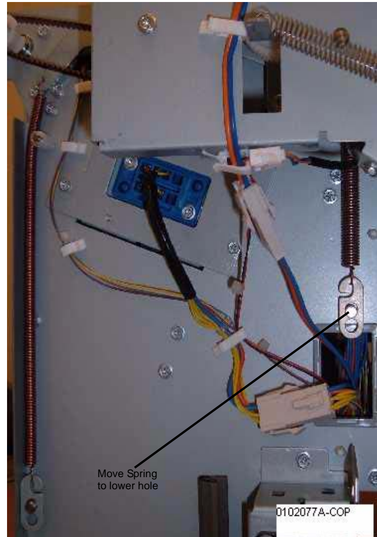
Figure 4 Adjusting the rear Spring tension
