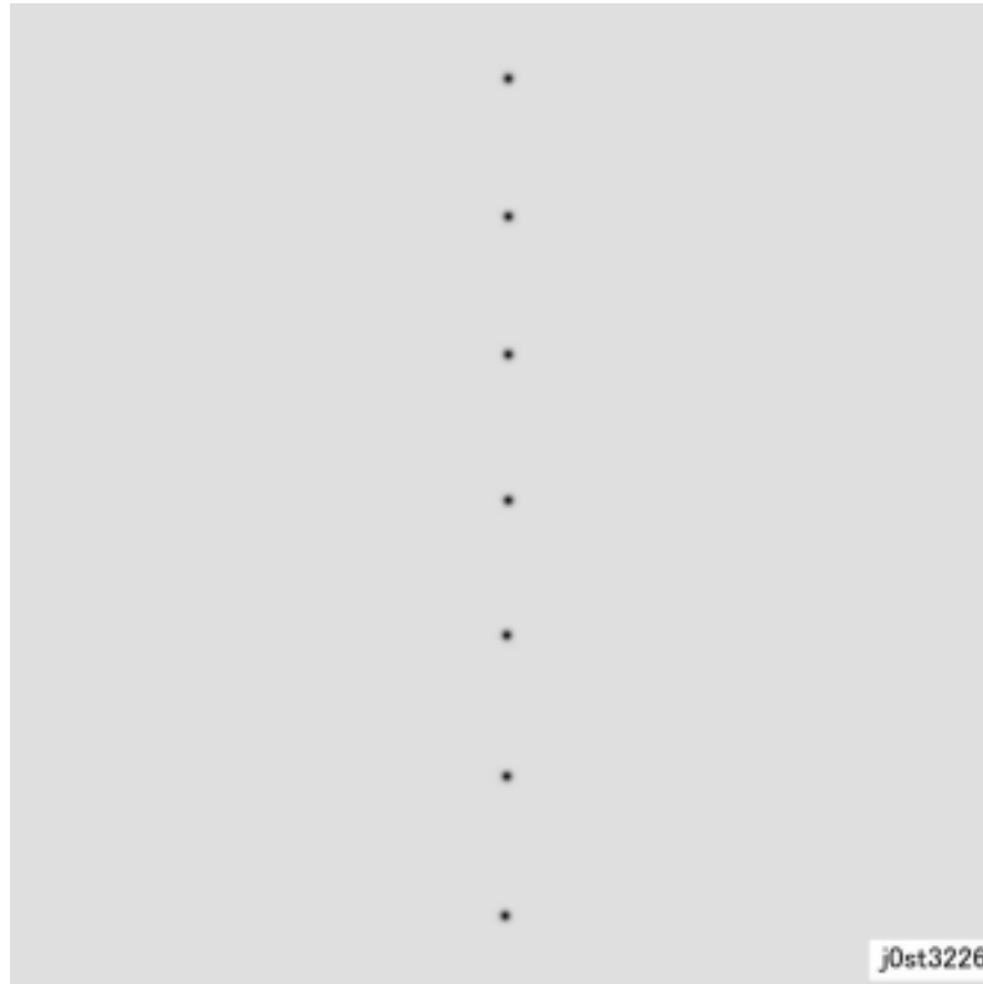
Figure 1 Regular Toner Contamination In Process Direction (Spots, Streaks, Bands etc.) Defect Sample (j0st3226)
