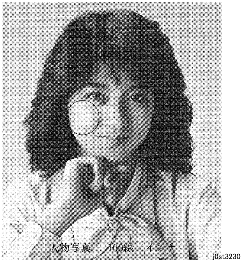
Figure 1 Gradation Jump In Text & Photo Mode For 100 Ipi Photo Originals Defect Sample (j0st3230)
