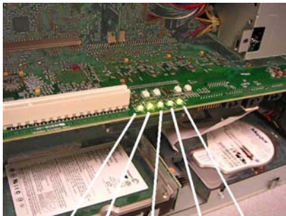
CR9 CR5 CR11 CR8 CR10 CD UP 3.3V PH 5V ON BLINK ON BLINK ON
