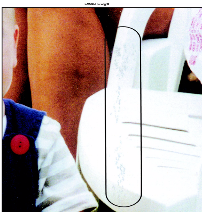
Figure 1 Newton Rings Defect Sample
