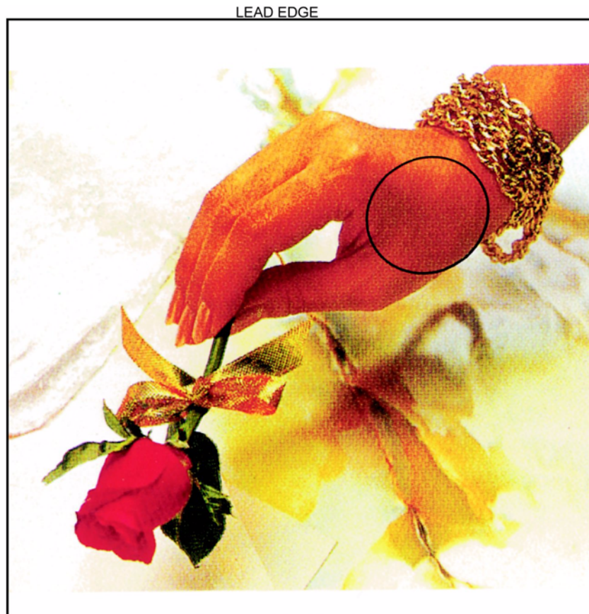
Figure 1 Moire Defect Sample
