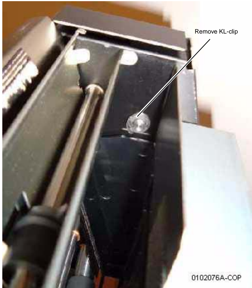
Figure 1 Removing the KL-clip
